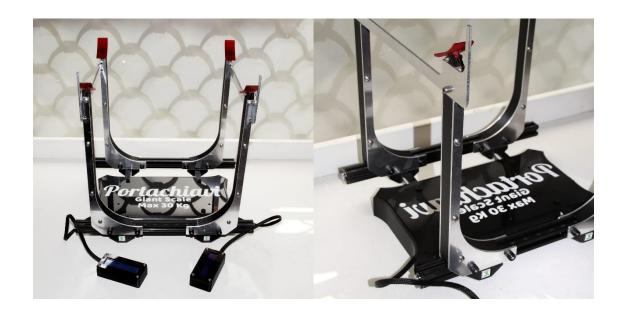
**Step 2**, slide the arms along the bar with rulers, now, you can adjust the arms to measure a plane, and fix the stopper on the leading edge of the plane. Every arm, have a 4 black nuts for screw and unscrew without tools, unscrew it for first slide, and fix when the scale are full mounted. The arms can be slide to make wider or narrow and adapt it to lot of gliders or airplanes.
