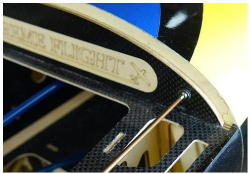
15. Secure your choice of tank to the tank tray over the carbon wing tube with Velcro or cable ties. We used the EF Flowmaster 34 ounce tank and fuel tubing along with an EF fuel dot. There is a laser cut hole in each side of the fuselage to install the EF fuel dot. You can also see the location of our receiver and the installation of the EF Multi-plugs in the sides of the fuselage in the following pictures.
