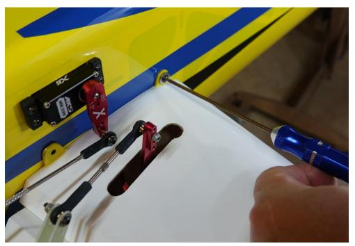
17. Slide the wing tube into the fuselage socket and slide the wings onto the tube. Connect the aileron servo extensions to the receiver (this is where the EF mutli-plug is of great benefit, please see picture).
