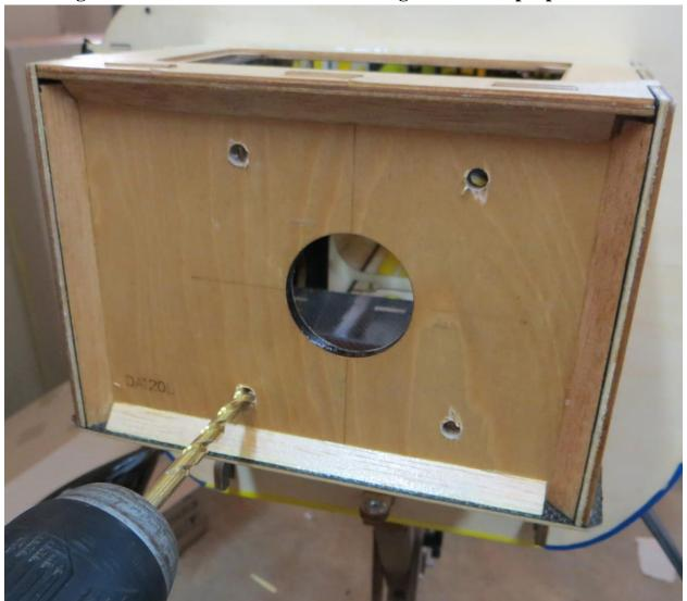
11. Install the DA-120 using the Blazing Star 1 inch mount and the single 3mm Delrin spacer provided with the mount. Be sure the spacer goes between the mount and plywood firewall, not against the engine. Secure using 1/4x20 bolts, washers and lock nuts (not included). Total distance from the front of the motor box to the rear of the spinner backplate is 7.35" or 187mm.
