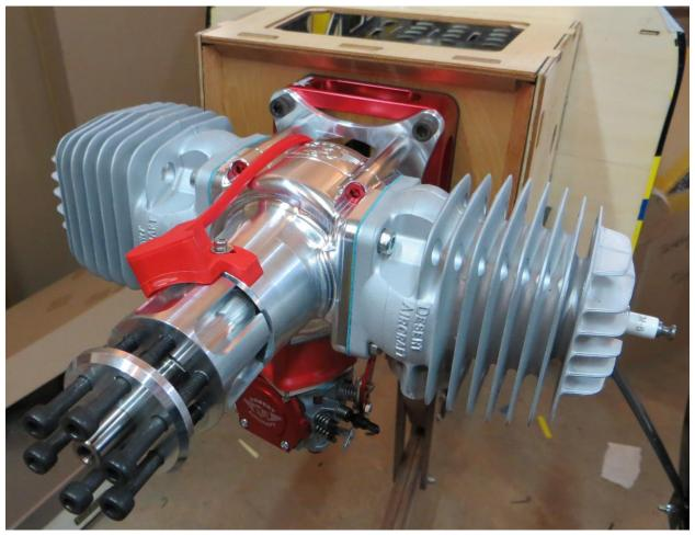
12. The following picture shows the location I mounted my throttle servo as well as the mufflers installed. Use a rotary tool to open the bottom of the cowl to fit the mufflers and to provide an exit for air. Notice I've also made a hole so that I can reach the choke lever easily with my finger. I find this easier than a dedicated choke servo installation and you save the weight of the servo and linkage. Some folks prefer to use a choke servo and that works great as well.
