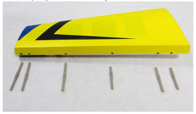
2. Install the control horns for the ailerons. \*\*\*PLEASE NOTE\*\*\* There are 2 different size control horns for the ailerons. The 2 longer sets are for the outboard aileron servos, the 2 shorter sets are for the inboard locations. Pay very close attention when separating and grouping the horns to be sure you are gluing the correct horns in the correct location!
