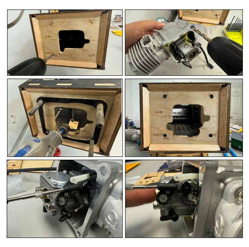
Mount your engine. Your can orient the bolts with the nuts to the either the front or rear, but you must use self-locking (Nyloc) nuts and you must use washers against the wood on the inside of the firewall. If you use the plastic spacers which are included with the Blazing Star mount, place the spacers between the mount and the wood firewall.
