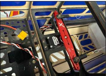
To terminate the cables at each end, you will use a ball link, a brass threaded end, and the small metal crimp tube. Thread the ball link onto the brass threaded end, and attach to the servo arm and control horn with screws, washers, locking nuts and cone spacers as applicable.
