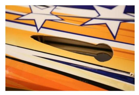
18. Remove the covering over these openings in the fuselage, for the wing tube, wing pins, and aileron servo wires.
