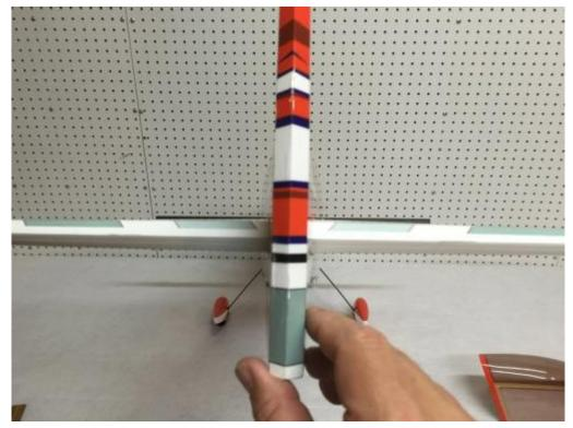
20. Once satisfied with the alignment, glue the horizontal stab in place by applying CA along the joint between the stab and fuse. Make sure to apply CA to the top and bottom of the stab, being careful not to get CA on the covering. Allow to dry.
