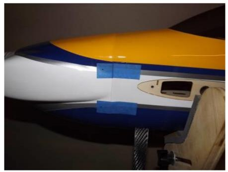
36. Remove the tape and secure the cowl with 4 of the included small wood screws that have the large heads.
