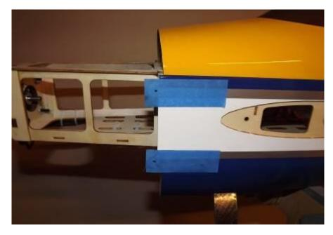
34. Install the canopy, roll the tape back and slide the cowl into position. Install the spinner backplate onto the motor shaft for reference and once satisfied with the cowl position roll the tape back into place and secure the cowl.
