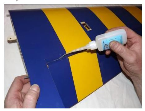
5. Before installing the aileron servo, take a minute and apply some CA to the servo tray and the anti-rotation pins.
