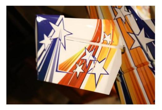
22. Test fit the right side elevator, and make sure the elevators are perfectly aligned. Sand the slot in the right side elevator as necessary to make the elevators align perfectly. Once the alignment is perfect, remove the right elevator apply epoxy to the joiner and slot as shown.
