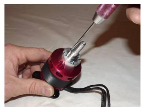
31. Install the motor with included 4mm screws into the pre-installed blind nuts.
