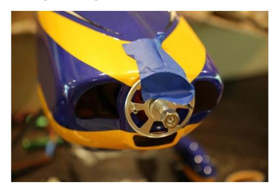
35. Use a 1/16" drill bit to drill a hole at the location of the dot on each piece of tape.
