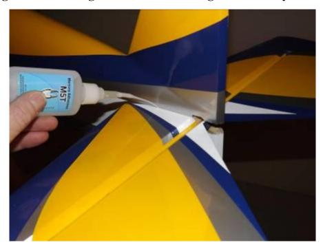
21. Install the left side elevator (with elevator joiner) as shown. Do not glue hinges yet.
