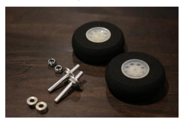
Place the wheel on the axle and secure with the wheel collar.
