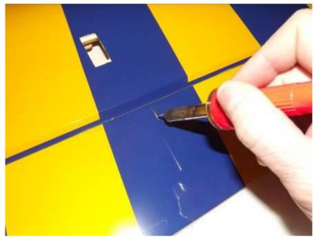
2. Use sandpaper to scuff the portion of the horn that will be inserted into the aileron. Glue the horn into the aileron as shown, making sure adequate epoxy is in the slot for a good bond. Wipe away any excess epoxy with a cloth soaked in denatured alcohol.
