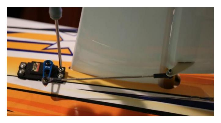
27. Locate the carbon fiber tailwheel assembly in the hardware package. Secure the tailwheel bracket to the bottom rear of the fuselage with the provided wood screws, making sure the pivot point of the assembly is over the hinge line of the rudder. It is a good idea to remove the set screws from the tailwheel assembly and apply blue Loctite to them, then re-install. Attach the tiller arm to the bottom of the rudder with the provided course pitch screw.
