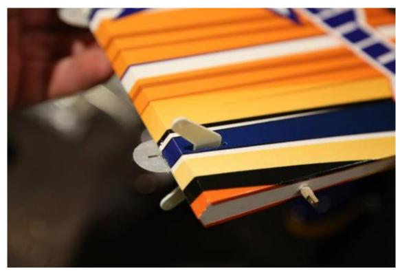
13. Check alignment of rudder hinges and slide rudder onto fuselage. Check for free swinging motion 45 degrees each way, and glue with thin CA glue as you did the aileron hinges.
