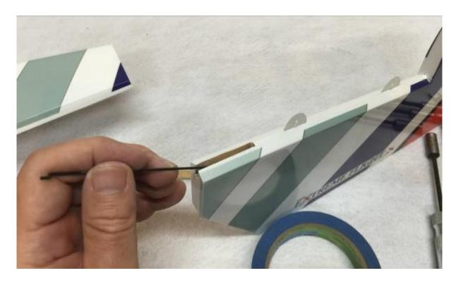
23. Re-install the right elevator, check alignment again, check for free movement 50 degrees up and down, glue elevator hinges with thin CA. Tape the elevators to the stab as shown to ensure perfect alignment while the epoxy cures.
