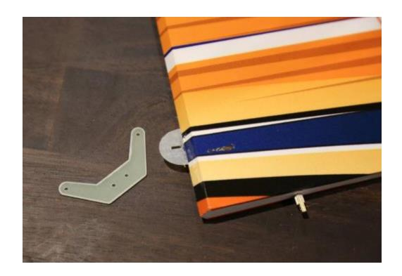
12. Scuff center of rudder control horn with sandpaper and glue into rudder with epoxy as shown. Allow to cure.
