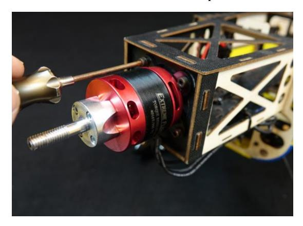
32. Install the ESC to the side or bottom of the motor box using zip ties or Velcro to secure the ESC. Connect the wires of the ESC and motor together.
