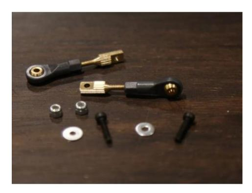
15. Using a piece of masking tape, tape the rudder so that it remains centered while you build the pull-pull cables. Screw the ball links and ends onto the rudder horn as shown, placing a washer on the ball-link side of the screw. Thread one of the brass tubes onto the pull-pull cable and loop the cable as shown. Pinch the tube with pliers to lock the cable. Add a drop of thin CA to the pinch. Repeat on other side.
