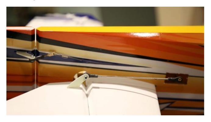
26. Install a 24" servo extension wire on the elevator servo, install into the fuselage as shown.
