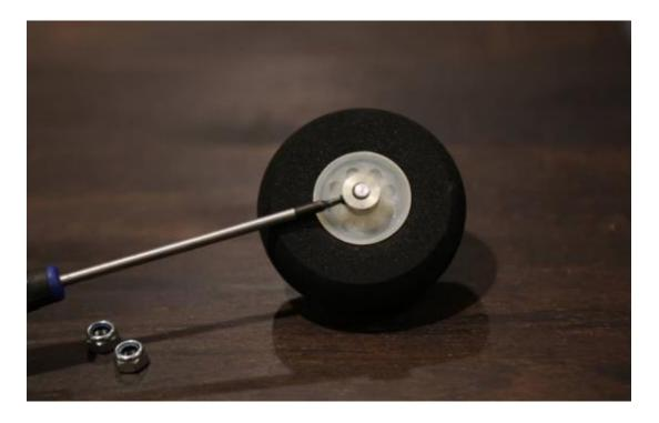
9. Place the threaded portion of the axle through the hole in the landing gear and attach the lock nut and washer onto the axle. NOTE: Note the LG has a tapered edge and a straight edge; make sure the straight edge faces the front. Slide the wheel pant into position over the axle and tighten the nut, making sure the wheel pant is positioned properly. Use the included metal wrench to hold the axle as shown, and tighten the nut securely.
