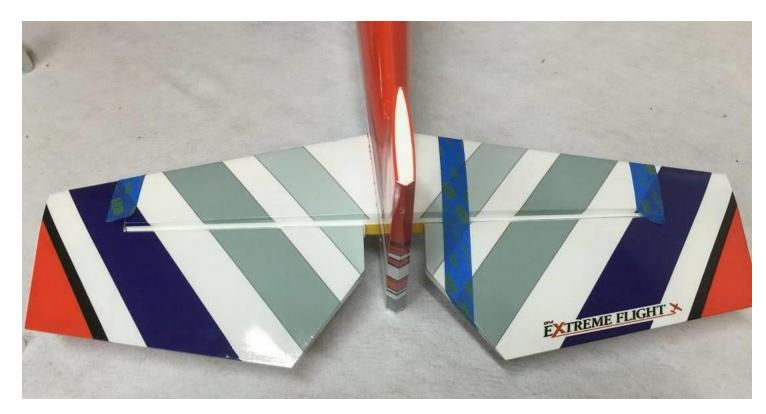
24. Remove the covering over the elevator control horn slot and elevator servo mount as shown.
