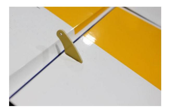
3. Flex the ailerons fully up and down, check for free action.
