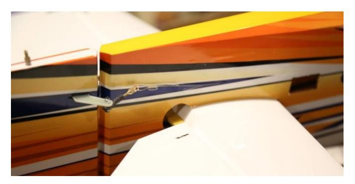
25. Scuff the elevator horn and install with epoxy as on the ailerons and rudder. Build and install pushrod as shown.
