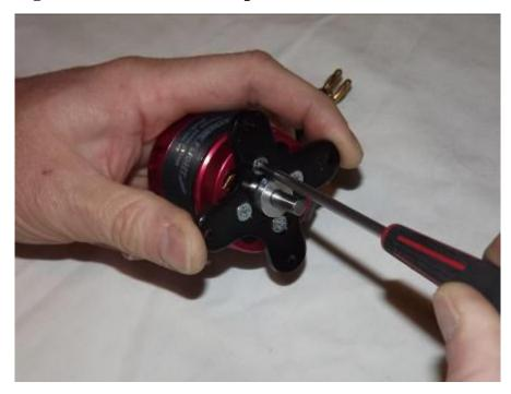
30. Secure the prop adapter using the 4 socket head cap bolts. Blue Loctite should be applied to each bolt.
