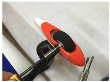
10. Secure the landing gear to the fuselage by inserting the 3mm bolt into a washer, through the carbon fiber gear and into the pre-installed blind nuts in the fuselage.
