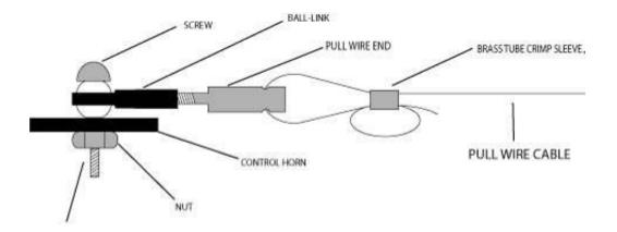
16. Mount the rudder servo as shown. Assemble the pull-pull cable ends as you did on the rudder end as shown. The cables should be taught, but not so tight as to cause drag on the servo.
