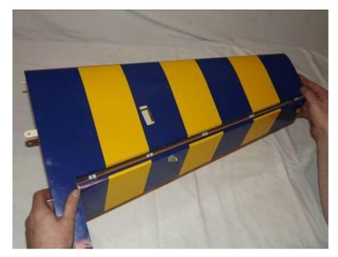
4. Making sure the aileron is properly aligned between the wing root and wing tip, hold the aileron fully deflected and apply a few drops of thin CA to each hinge. Flip the wing over and repeat.
