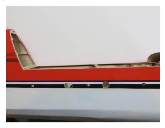
19. Insert the stabilizer into its slot and the carbon fiber wing tube into the fiberglass sleeve. Use a ruler to insure that the stabilizer is centered in its slot and compare the stabilizer to the wing tube to make sure it is properly aligned. Sand or shim the slot if necessary to ensure proper alignment.
