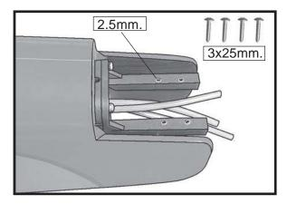
$\Box$  5) Bolt the engine to the engine mount using the four machine screws. Double check that all the screws are tight before proceeding.
