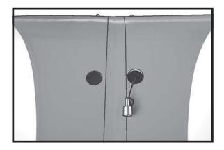
□ 3) Attach servo lead to the aileron servo. Attach the string to the servo lead and carefully thread it though the wing. Once you have thread the lead throught the wing, remove the string so it can use for the other servo lead.
