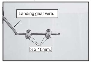
$\Box$  6) Reinstall the gear wire and install the straps using the four 3 x 10mm wood screws. Tighten the screws completely to secure the gear wire in place.
