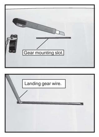
□ 3) The landing gear wire is held in place using two nylon landing gear straps and four 3mm x 10mm wood screws.
