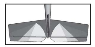
$\Box$  4) With the stabilizer held firmly in place, use a pen and draw lines onto the stabilizer where it and the fuselage sides meet. Do this on both the right and left sides and top and bottom of the stabilizer.
