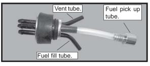
When the stopper assembly is installed in the tank, the top of the vent tube should rest just below the top surface of the tank. It should not touch the top of the tank. □ 5) Test fit the stopper assembly into the tank. It may be necessary to remove some of the flashing around the tank opening using a modeling knife. If flashing is present, make sure none falls into the tank.
