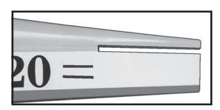
$\Box$ 1) Using a ruler and a pen, locate the centerline of the horizontal stabilizer, at the trailing edge, and place a mark. Use a triangle and extend this mark, from back to front, across the top of the stabilizer. Also extend this mark down the back of the trailing edge of the stabilizer.
