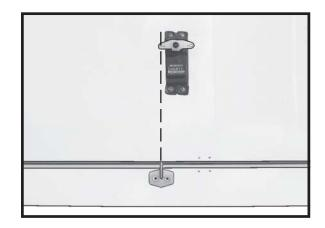
□ 6) Thread one nylon adjustable control horn onto each aileron control rod. Thread the horns on until they are flush with the ends of the control rods.
