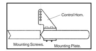
□ 4) Using a 1mm drill bit and the control horns as a guide, drill the mounting holes through the aileron halves.
