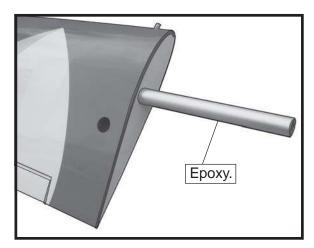
Carefully slide the two wing halves together and firmly press them together, allowing the excess epoxy to run out. There should not be any gap in the wing halves. Use rubbing alcohol and a paper tower to clean up any excess epoxy.
