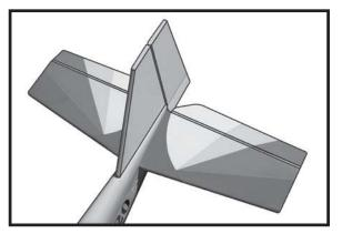
□ 3) While holding the vertical stabilizer firmly in place, use a pen and draw a line on each side of the vertical stabilizer where it meets the top of the fuselage.
