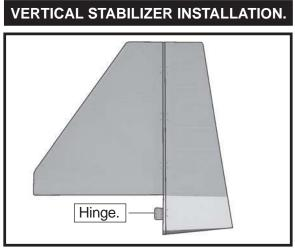
□ 1) Using a modeling knife, remove the covering from over the precut hinge slot cut into the lower rear portion of the fuselage. This slot accepts the lower rudder hinge.
