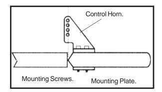
$\Box$  3) Using a 2mm drill bit and the control horns as a guide, drill the mounting holes through the elevator halves.
