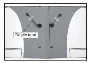
□ 5) Reinstall the servo into the servo mount and secure the servo inplace using the wood screws provided with you radio system.
