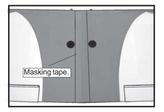
□ 3) Peel off the backing from the self adhesive covering strip. Apply the strip to the centre section of the wing starting from the bottom trailing edge. Wrap the strip all the way around the wing until it meets the trailing edge again. Trim off any excess strip.
