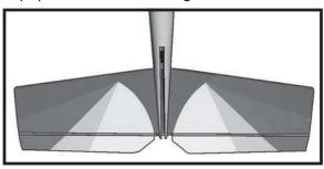
□ 8) After the epoxy has fully cured, remove the masking tape or T-pins used to hold the stabilizer in place. Carefully inspect the glue joints. Use more epoxy to fill in any gaps that may exist that were not filled previously and clean up the excess using a paper towel and rubbing alcohol.
