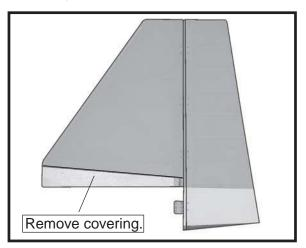
When cutting through the covering to remove it, cut with only enough pressure to only cut through the covering itself. Cutting into the balsa structure may weaken it.
