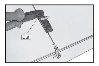
$\square$  8) Make a 90-degree bend at the mark and cut off the excess wire leaving 10mm past the bend.
