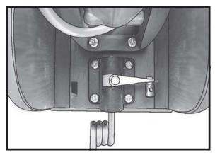
Install the pushrod wire as shown.
