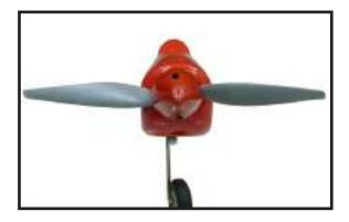
The propeller should not touch any part of the spinner cone. If it does, use a sharp modeling knife and carefully trim away the spinner cone where the propeller comes in contact with it.
