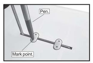
$\Box$  5) Remove the two straps and the gear wire. Drill four 1.5mm pilot holes into the wing for the wood screws.
