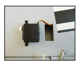
9) Set the aileron servo in place and use a Phillips screw driver to install it with four wood screws.
