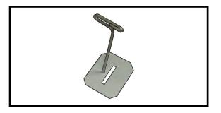
2) Remove each hinge from the wing panel and aileron and place a T-pin in the center of each hinge. Slide each hinge into the wing panel until the T-pin is snug against the wing panel. This will help ensure an equal amount of hinge is on either side of the hinge line when the aileron is mounted to the aileron.
