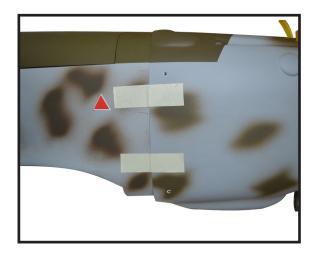
2) Use a drill and drill bit to drill the holes for the cowl mounting screws. Make sure the cowl position is correct before drilling each hole.
