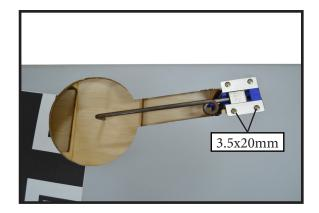
2) Install servo for Retractable landing gear.
