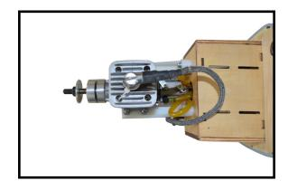
Blow through one of the lines to ensure the fuel lines have not become kinked inside the fuel tank compartment. Air should flow through easily.
