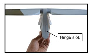
3) While holding the vertical stabilizer firmly in place, use a pen and draw a line on eachside of the vertical stabilizer where it meets the top of the fuselage.
