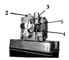
(1)风门,冷启动时使用;Choke Arm (The Choke Arm is used under the circumstance of cold start-up.);(2)油门;Throttle;(3)总速调节螺丝;Idle Adjustment Screw;(4)低速油针;Low-speed Needle;(5)高速油针;High-speed Needle;
