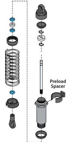
The model's ride height can be adjusted by adding or removing the clip-on, spring preload spacers. Adjust the ride height so that the suspension arms are slightly above being parallel to the ground. Observe how the model handles in turns. Proper setup will add stability and help prevent spin outs. Experiment with different springs and shock oils to find what works best for your current track conditions.
