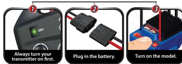
• Always use new or freshly charged batteries for the radio system. Weak batteries will limit the radio signal between the receiver and the transmitter. Loss of the radio signal can cause you to lose control of your model.
