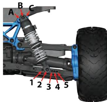
The suspension of your model has been set up for off-road performance (position 2 on the front suspension arms and position 3 on the rear suspension arms). If you plan on driving on hard surfaces, the following changes should be made:
