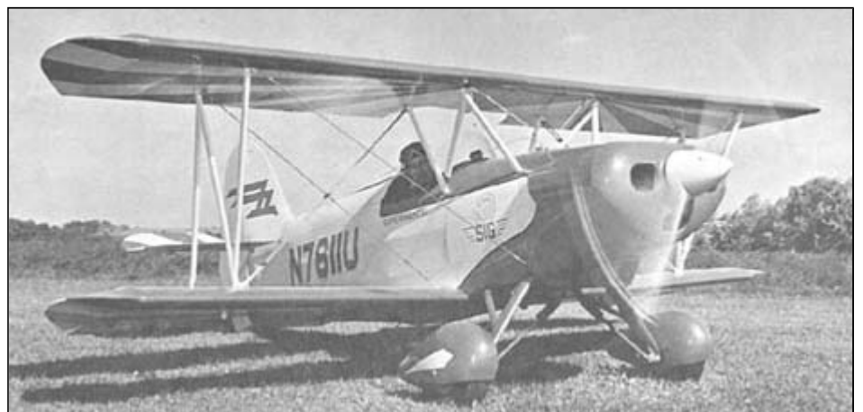
An 108 HP Lycoming coupled with light weight produces a snappy aerobic performer
