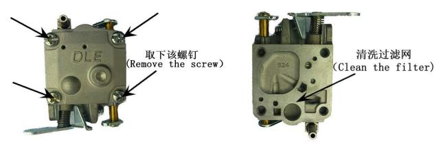
NOTICE: The carburetor fuel screen should be cleaned periodically also. Carefully remove the pump cover (inlet side of the carburetor), gasket and pump membrane. The screen will be visible and can be cleaned after careful removal.
