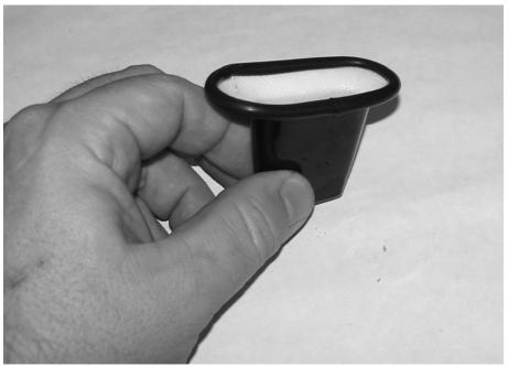
18. Slide the fairings over the landing gear and against the sides of the fuselage. You may need to open the hole in the fairing slightly with a rotary tool bit for proper fit. Use a pencil to mark the location of the bottom of the fairing on the landing gear and then remove the fairing.
