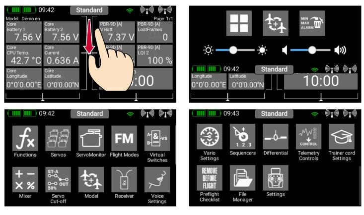
There is no need to press firmly, as the capacitive touch-screen simply responds to touch, like all modern smartphones. The symbols in the Main menu are arranged in order of importance.
