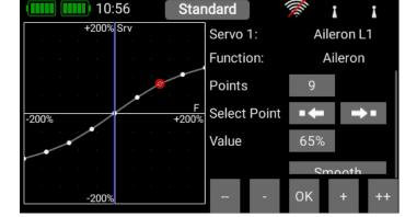
Here you will find the assigned servos again. Up to eight servos can be assigned to each function. As already mentioned in the **Assistant**, the travel and end-points of each servo can be adjusted separately here. Any adjustments you make to a servo at this point have no influence on the settings of the same servo if it is also assigned to another function. This provides a simple means of mixing in aircraft with multi-flap wings, delta wings and V-tails.
