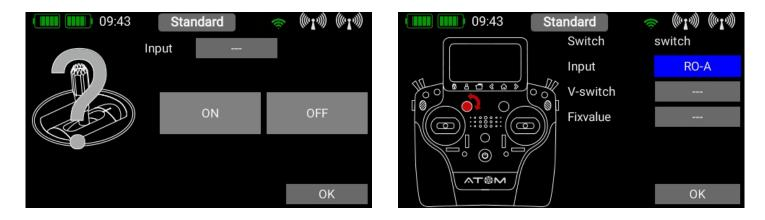
A further alternative is to define a fixed value - **On** or **Off**. This is necessary, for example, if you only wish to assign a switching threshold to one linear control. In this case select one transmitter control as fixed value, and define a linear control for the other transmitter control.
