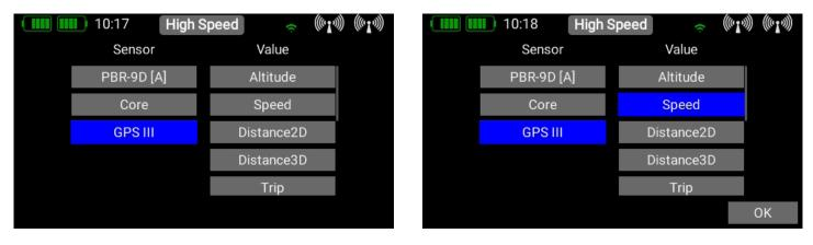
The left-hand column shows all the connected sensors, while the right-hand column shows all the values which these sensors supply. The **P**<sup>2</sup>**BUS** is an in-house development, and is capable of transmitting up to **255 sensors each with 32 individual values** – and at a speed of up to **800 values per second**!
