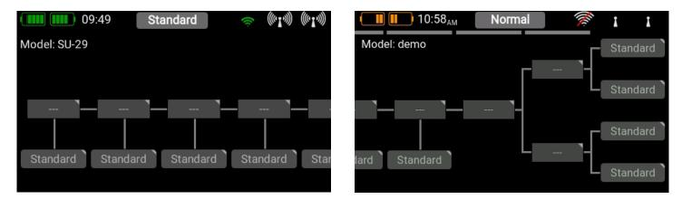
The most important thing to know at this point is that the **ATOM** prioritizes the flight modes. Priority runs from left to right, i.e. the flight modes in the left-hand tree diagram have the highest priority, and those on the right the lowest priority. Even when the flight mode structure is complex, this means that you can, for example, overrule all other switch positions with a single switch, returning you very quickly to "normal" flight mode.
