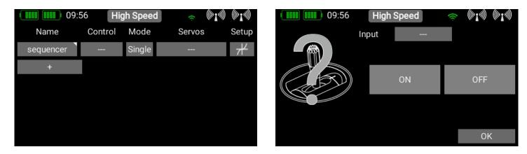
The transmitter control can be either a switch or a linear control. In both cases you can set the desired switching points and the switching direction. Please note that the green range covers the sequencer running **forward**, the red range the **reverse** range. More on this later when we discuss the method of setting travel points.
