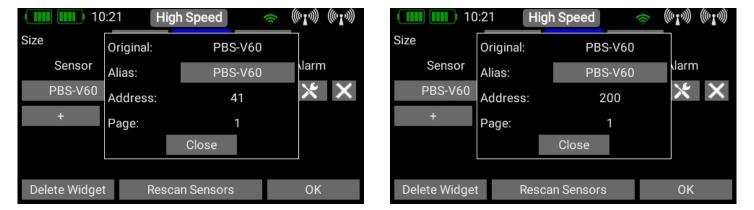
• Now connect the next sensor, and carry out another **Sensor Rescan** process. Press + to accept the second sensor into the system.
