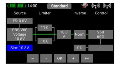
If the telemetry control is above the set value of 11.0V, 0% is added to the throttle servo, i.e. the throttle channel behaves in the usual way.
