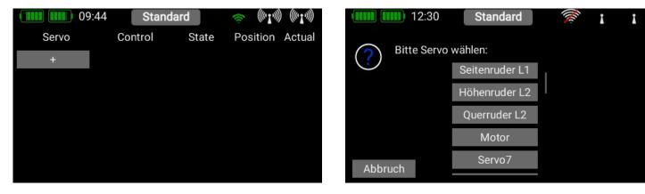
First select a **transmitter control** by briefly pressing the blank field (three dashes) under Control; press Control again at the next screen. You can now select a switch or linear control as transmitter control by operating it.
