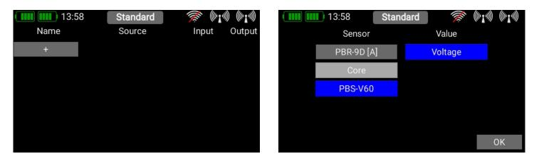
In this example the **PBS-V60** voltage sensor is to be used to reduce motor power if the voltage of the flight battery falls to a dangerous level. You can rename the telemetry control under the **Name** field.
