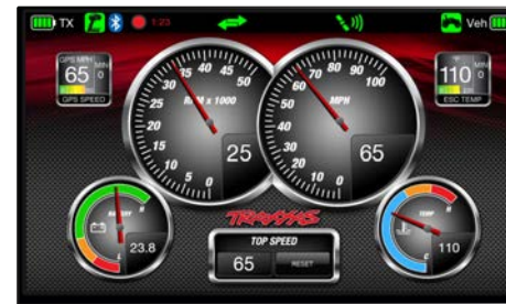
The customizable Traxxas Link dashboard delivers real-time rpm, speed, temperature, and voltage data.
