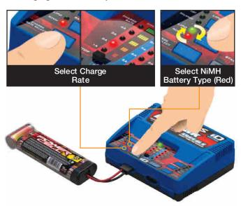
Press and hold the Start button(s) for 1 second. The charger will play a tone, indicating that charging has started. Press once to stop. The charger will play a tone, indicating that charging has been canceled. The charge progress LEDs will light as the battery charges.
