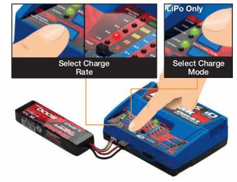
Press and hold the Start button(s) for 1 second. The charger will play a tone, indicating that charging has started. Press once to stop. The charger will play a tone, indicating that charging has been canceled. The charge progress LEDs will light as the battery charges.
