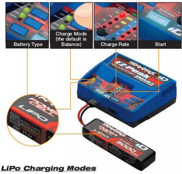
Change your LiPo charging mode if desired. The default setting for iD LiPo batteries is Balance Charge.
