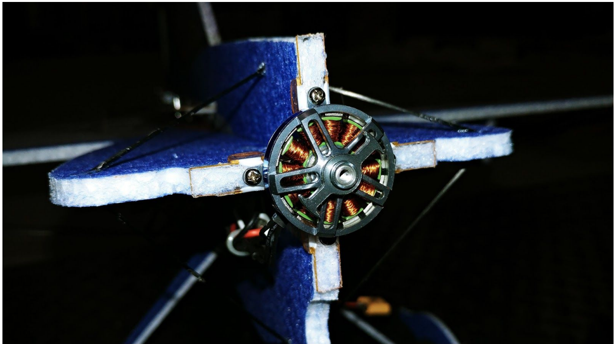
Shown above is the motor mounted to the provided motor mount.
