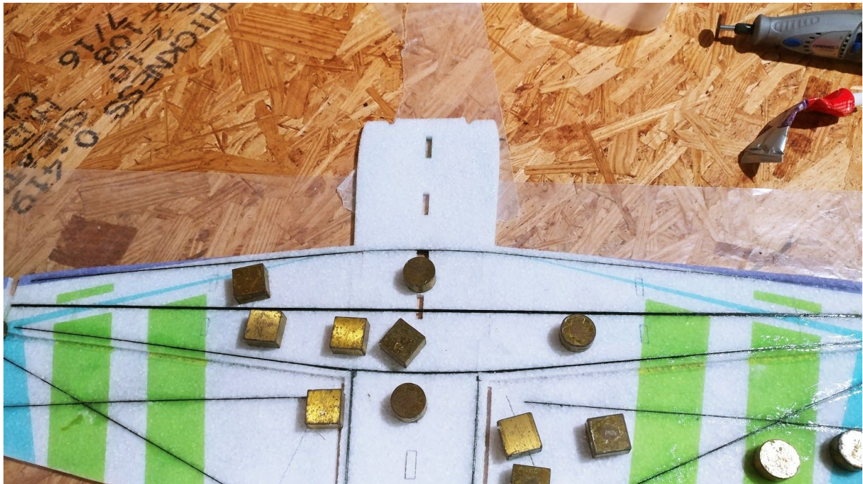
Wing bracing shown above. The center wing spar is the supplied carbon fiber square stock.
