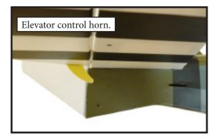
1) Thread one clevis and M2 lock nut on to the elevator control rod. Thread the clevis on until it is flush with the end of the control rod.
