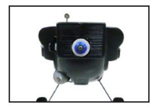
2) Install the muffler and muffler extension onto the engine and make the cutout in the cowl for muffler clearance. Connect the fuel and pressure lines to the carburetor, muffler and fuel filler valve. Secure the cowl to fuselage using the M3x10mm screws.
