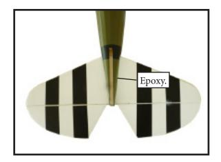
4) Slide the vertical stabilizer back inplace. Using a triangle, check to ensure that the vertical stabilizer is aligned 90° to the horizontal stabilizer.
