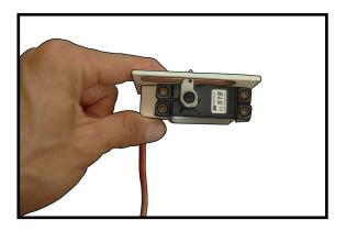
2) Use drill bit in a pin vise to drill the mouting holes in the blocks.
