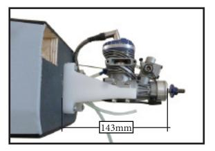
2) Use a pin drill and 4mm drill bit to drill a small indentation in the mount for the engine mounting screw.
