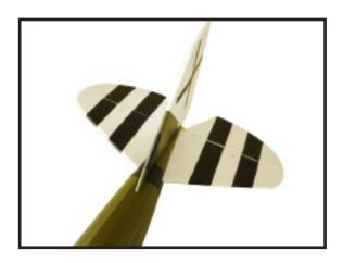
5) When you are sure that everything is aligned correctly, mix up a generous amount of Flash 30 Minute Epoxy. Apply a thin layer to the mounting slot and to bottom of the vertical stabilizer mounting area. Apply epoxy to the bottom and top edges of the filler block and to the lower hinge also. Set the stabilizer in place and realign. Double check all of your measurements once more before the epoxy cures.
