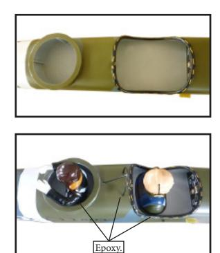
4) Position the windshield onto the fuselage. Trace around the windshield onto the fuselage using a felt-tipped pen. Cut and remove the covering from between the lines drawn, and glue the windshield to the fuselage using epoxy or a special canopy glue.
