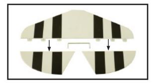
2) Carefully remove the elevator from one of the horizontal stabilizer panels. Note the position of the hinges.
