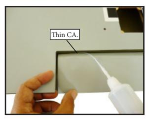
5) Turn the wing panel over and deflect the aileron in the opposite direction from the opposite side. Apply thin C/A glue to each hinge, making sure that the C/A penetrates into both the aileron and wing panel.
