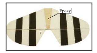
7) When you are sure that everything is aligned correctly, mix up a generous amount of 30 Minute Epoxy. Apply a thin layer to the top and bottom of the stabilizer mounting area and to the stabilizer mounting platform sides in the fuselage. Slide the stabilizer in place and realign. Double check all of your measurements once more before the epoxy cures. Hold the stabilizer in place with T-pins or masking tape and remove any excess epoxy using a paper towel and rubbing alcohol.
