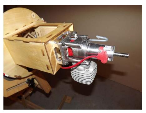
49. Next, install the throttle servo in the pre-cut servo hole located in the bottom of the motor box. Locate the 2mm pushrod and white ball links to fabricate the throttle linkage. If using a pipe you will need to add 3/8" hardwood rails to raise the servo.
