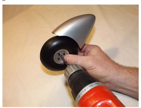
44. Insert the threaded portion of axel through the spat, then mount the axel and spat onto the landing gear. Secure the axel to the landing gear with a washer and nylon lock nut. Position the spat as desired and mark the location for the blind nut using the pre-drilled hole in the aluminum gear as a guide. Install the 3mm blind nut and secure the spat with a 3mm washer and hex nut.
