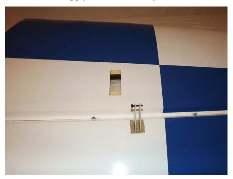
25. Attach a 6" servo extension to your servo and secure with thread or heat shrink tubing. Use the manufacturer supplied mounting hardware to install the servo with the output shaft toward the leading edge of the wing. Electronically center the servo.
