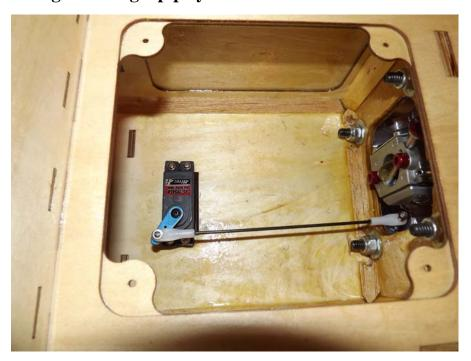
Note: If you are using a DA-50 or DA-60 you may need to rotate the carburetor 180 degrees so that the throttle arm is facing the bottom of the motor box. Also, it's a good time to coat the inside of the motor box with thinned epoxy.
