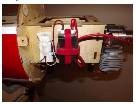
51. Install the tank of your choice-- for our build we used a Dubro 24 oz tank. Make sure to use a gas compatible stopper and tubing for all plumbing. Use Velcro Straps or nylon cable ties to secure the tank to the tank tray. The tank should butt up against the wing tube. Also, install foam between the tank and tray to protect against vibration.
