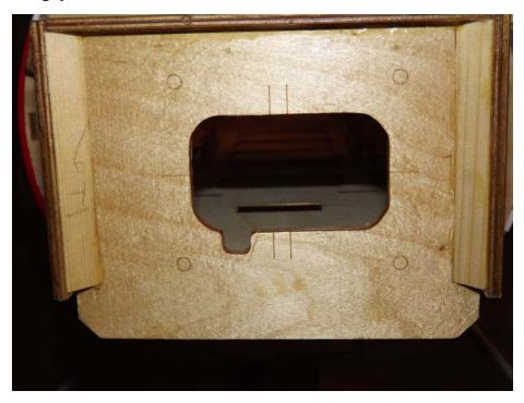
47. If using a different engine, tape the manufacturers mounting template onto the front of the firewall making sure to align the horizontal and vertical lines on the template with the laser scribes lines on the firewall. Be sure to use the offset line to the right of the vertical center line in order to accommodate for the motor offset due to the built in right thrust angle in the motor box.
