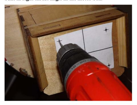
48. Use the recommended mounting bolts to mount the engine to the firewall making sure to use large washers behind the firewall to distribute the load. Use standoffs to ensure the motor extends 6.32 inches (160mm) from the firewall to the engine thrust washer.
