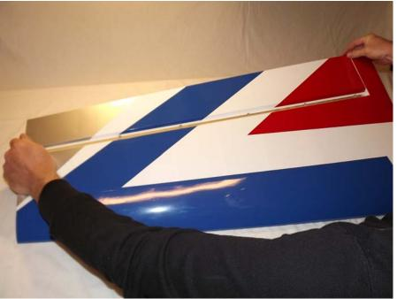
Note: Before moving to the next step – it would be a good time to seal the hinge gap with a strip of Ultracote or Blenderm tape. Be sure to fully deflect the control surface when sealing the gap to allow for full deflection once the gap is sealed.
