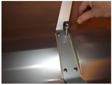
42. Attach the landing gear fairings with silicon glue.
