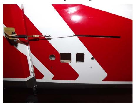
58. Attach 36 inch servo extensions to each elevator servo. If you plan to remove the stabs for transport, you will need 48 inch extensions. Slide the stab halves onto the carbon fiber stab tube and secure with a 3mm bolt and washer inserted through the mounting tabs and into the pre-mounted blind nuts. Make sure to use a drop of blue Loctite on these bolts.
