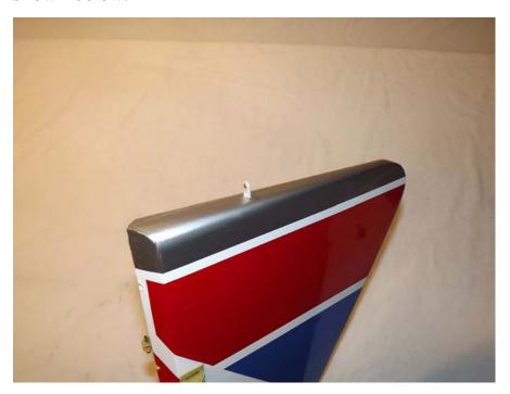
33. Next install the rudder hinges using the same procedure as with the Ailerons and Elevators. Use painters tape to hold the rudder in place while the epoxy dries.
