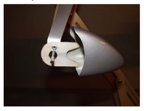
45. Install one wheel collar on the axel first in order to center the wheel on the axel. Next, slide the wheel onto the axel and secure the wheel with the second wheel collar. Repeat this process for the remaining wheel and spat.
