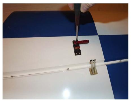
26. Use the recommend 1.50" SWB servo arms and attach 2 ball links onto the titanium turnbuckle pushrod. Secure the pushrod to the control horns and servo arm using the supplied 3mm bolts, washers, and nylon insert locknuts as shown in the picture below. As always, use blue Loctite on ALL bolts!
