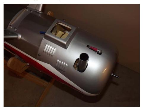
56. Once you're satisfied with the fit of the cowl, add some thick CA or Epoxy to the intersection of the cowl and plywood cowl ring. Slide the cowl into position and secure with 4 x 3mm bolts and bonded washers through the pre-drilled holes in the cowl. (2 per side)
