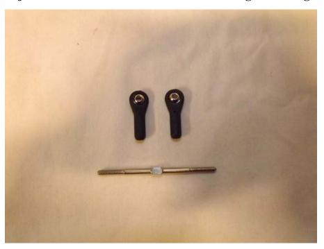
20. As shown in the picture below, secure one end of the ball link to the servo arm using a 3mm socket head cap screw, washer and nylon insert locknut. If using the SWB arms, you will need to drill out the hole to accept the 3mm bolt. Secure the other end of the ball link to the control arm with a 3mm bolt, 2 washers, and nylon insert locknut being careful not to over-tighten and damage the control arms.
