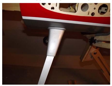
43. Locate the 2 axles, 2 locking nuts, 2 washers, 2 wheels, 4 wheel collars and 2 wheel spats. Center the wheel on the spat and drill a hole for the axel. If flying on a grass field you may want to drill the about 1/4" below center to allow the spat to be positioned slightly higher than center to prevent it from making contact with the ground.
