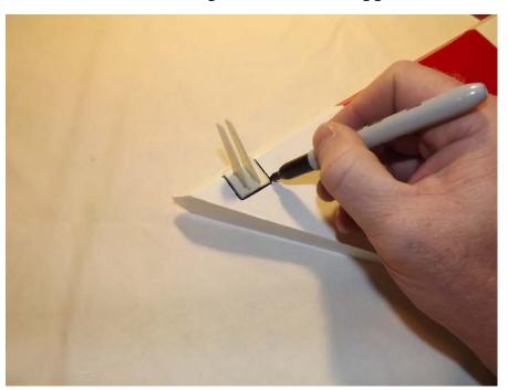
4. Remove the horn assembly and use a #11 blade to remove the covering from inside the ink line you traced around the control horn base.
