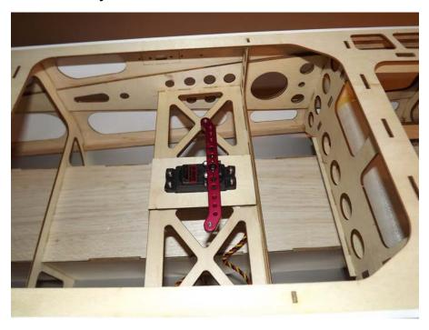
39. Next, install the pull-pull rudder cables. Assemble one end of the linkage by inserting the pull-pull cable into one of the aluminum crimp tube, through the hole in the brass pull-pull fitting and back through the crimp tube. Loop the cable back through the crimp tube a second time and crimp with side cutters.
