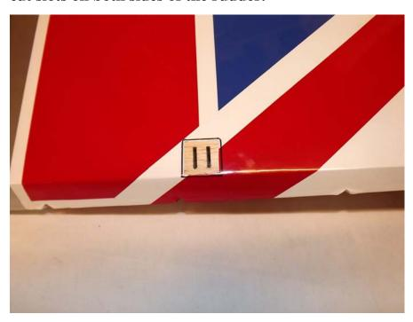
30. Mix a generous batch of epoxy and completely fill the two slots as well as the areas on control horns and base plates that will glue into both sides of the rudder.
