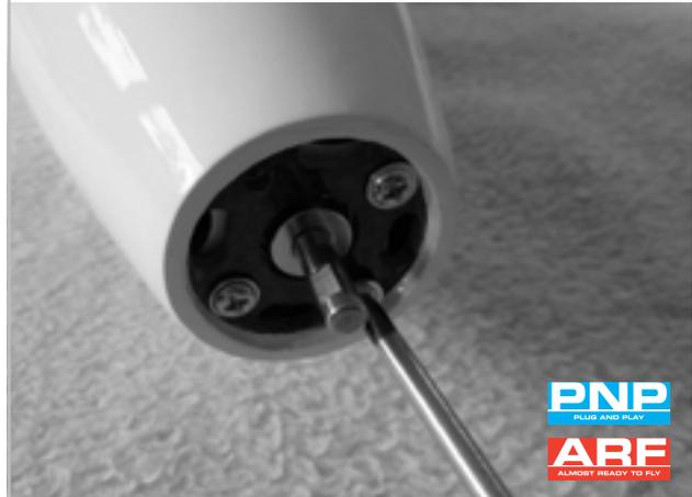
Install the motor and use threadlock.
