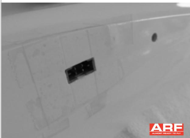
Cover the area around the MPX connector with clear tape.
