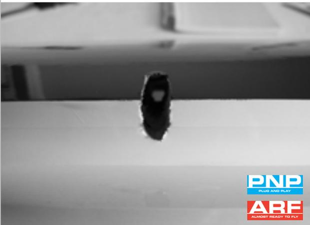
Enlarge the hole at the exit in the direction to the hinge, that the linkage will not be blocked when the flaps are full driven.
