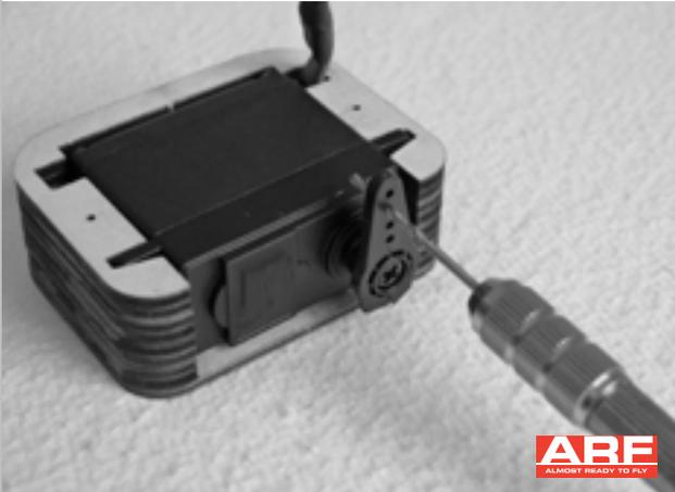
Remove any arm that may interfere with the operation of the servo. Enlarge the second hole to 1,6mm.
