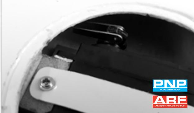
Attach the clevis to the servo horn.
