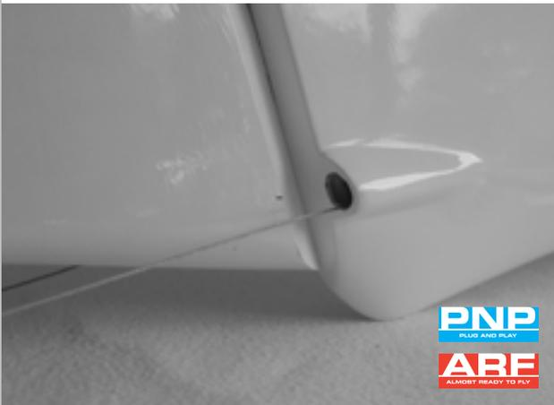
Mark at the rudder the position of the rudder horn.
