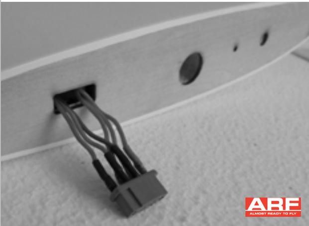
Solder a Multiplex connector to the servo cable.
