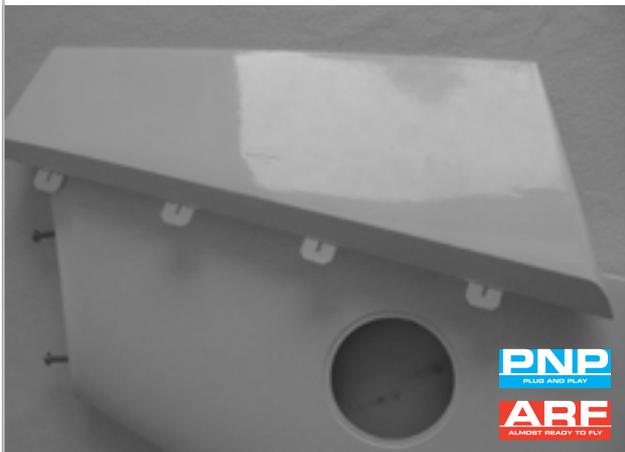
Install four cyano hinges in the rudder.
