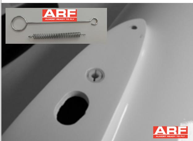
Glue the sleeve of the multilock (optional) flush with UHU Endfest 300 into the fuselage. Make sure to sand the outside of the sleeve beforehand. If you do not install multilock quick-release fasteners, the ARF model comes with a tensioning spring and mounting aid so that you can mount the surfaces evenly on the fuselage.
