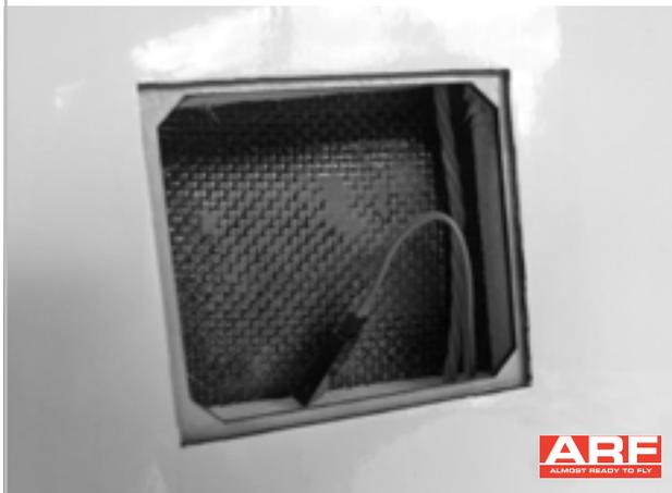
Sand the bottom of the wing and the servo mount thoroughly. Pull the cable of the aileron servo and a female servo connector through this part of the wing.
