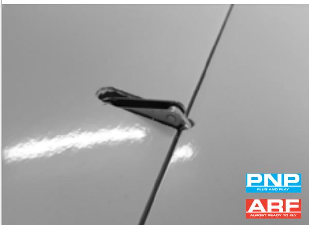
Fix the flap to the maximum up position (Speed position). Mount the clevis to the rudder horn.
