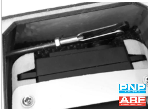
Adjust the servo to the maximum throw with the servo horn facing to the leading edge of the wing. Fix the servo in the mount using the plastic strip and self tapping screws.
