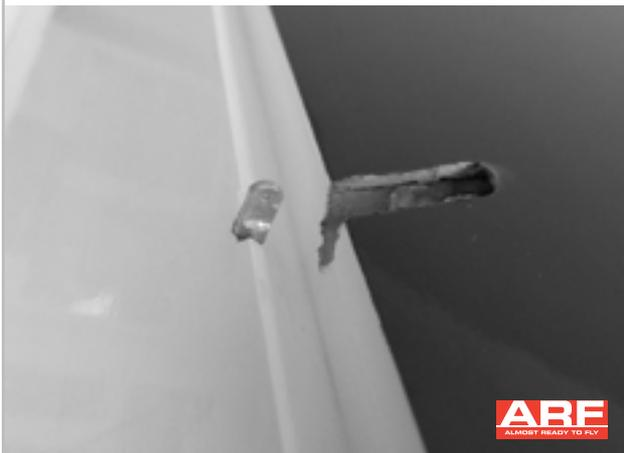
Glue the rudderhorn with epoxy. The rudderhorn should stick nearly to the flat area in the flap.
