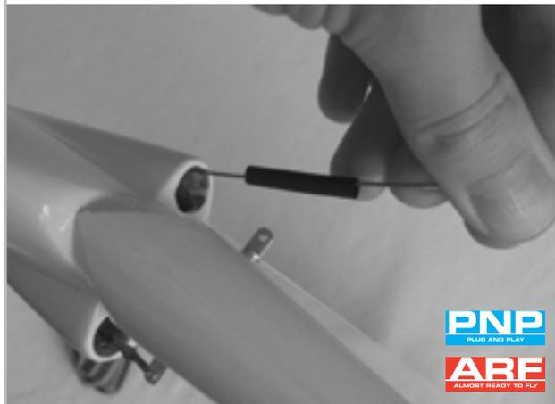
Pull a piece of 3mm Heatshrink tube on the cable.
