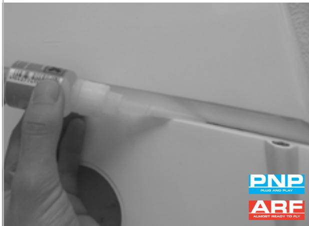
Attach the rudder to the fuselage and apply from both sides thin CA to the hinges. Let the CA cure for 30 minutes and don't use activator. Don't use medium or thick CA as this will not soak in the hinges.
