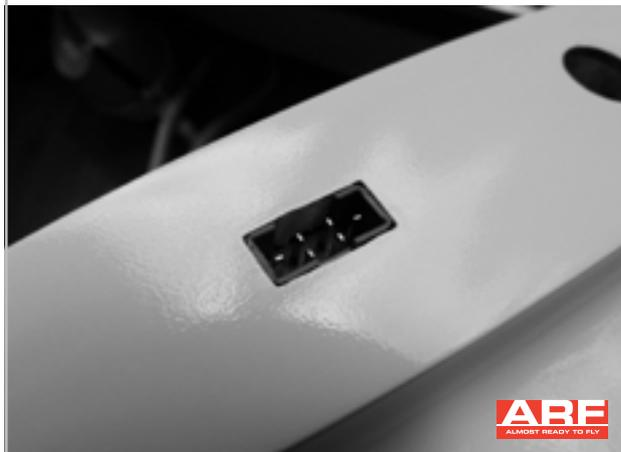
Route the cable harness through the fuselage and glue it flush with the wing cheeks of the fuselage. Please sand the connector before you start gluing.
