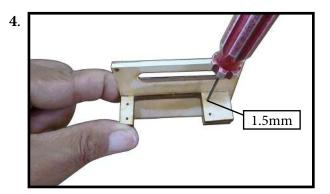
Apply 2-3 drops of thin C/A to each of the mounting holes. Allow the C/A to cure without using accelerator.
