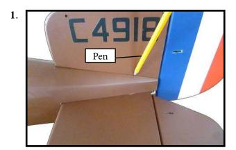
Using a modeling knife, remove the covering from over the precut hinge slot cut into the lower rear portion of the fuselage.
