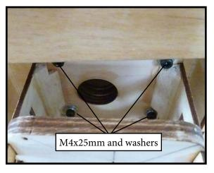
Attach the motor mount to the front of the electric motor box using four 4mm blind nut, four M4x20mm hex head bolts to secure the motor. Please see picture shown.
