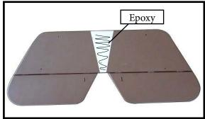
When you are sure that everything is aligned correctly, mix up a generous amount of 30 Minute Epoxy. Apply a thin layer to the top and bottom of the stabilizer mounting area and to the stabilizer mounting platform sides in the fuselage. Slide the stabilizer in place and realign. Double check all of your measurements once more before the epoxy cures. Hold the stabilizer in place with T-pins or masking tape and remove any excess epoxy using a paper towel and rubbing alcohol.
