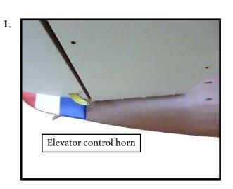
Thread one clevis and M2 lock nut on to each elevator control rod. Thread the horns on until they are flush with the ends of the control rods.
