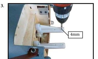
The fire wall has the location for the throttle pushrod tube (pre-drill).
