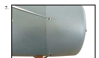
Install the muffler and muffler extension onto the engine and make the cutout in the cowl for muffler clearance. Connect the fuel and pressure lines to the carburetor, muffler and fuel filer valve. Secure the cowl to fuselage using the M3x10mm socket head screws. Putting a small length of silicon fuel tube under the head of the screw helps with vibration.
