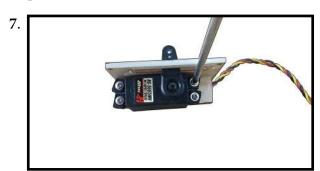
Apply 1-2 drops of thin C/A to each of the mounting tabs. Allow the C/A to cure without using accelerator.
