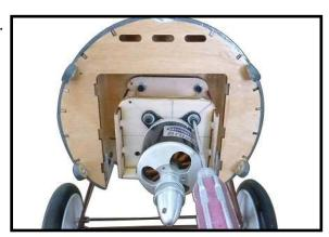
electric motor box using four 4mm blind nut, four M4x20mm hex head bolts to secure the motor. Please see picture shown.
