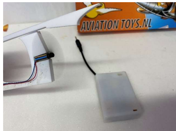
019. Make sure you have attached the prop correct, charge the system for 1 or 2 seconds and check the wind gets blown towards the back of the plane.
