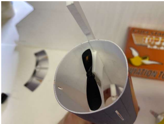
034. You can center the tube when you look inside the "tube" and use the line for reference.
