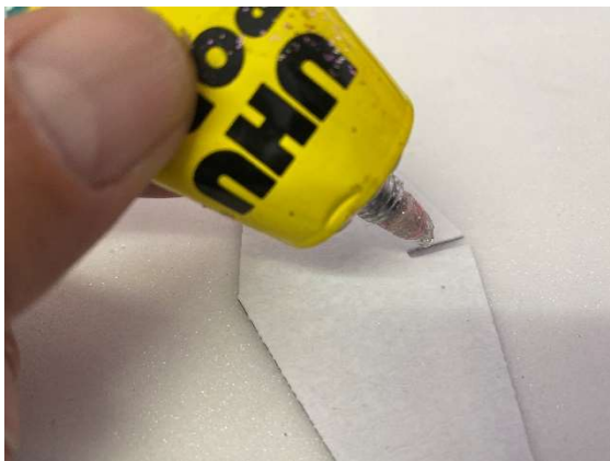
060. Apply glue in the gap of the stabiliser.
