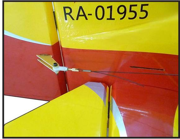
Loop the cable back through the brass swage tube and tighten the second loop through the brass swage tube as shown.
