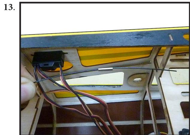
Thread cable through the threaded coupler hole, and back through the brass swage tube as shown.
