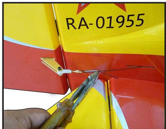
Cut off excess cable as shown.
