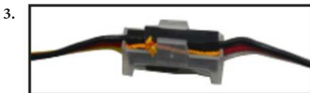
Fasten the pull string from the servo hole to the male plug of the servo extension.
