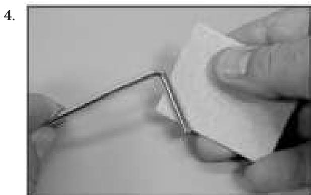
Fit the joiner wire into the elevator halves.
