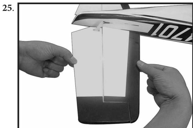
Flex the control surface through its range of motion a few times to break-in the hinges. This will reduce the initial load on the servo when the surface is first actuated.
