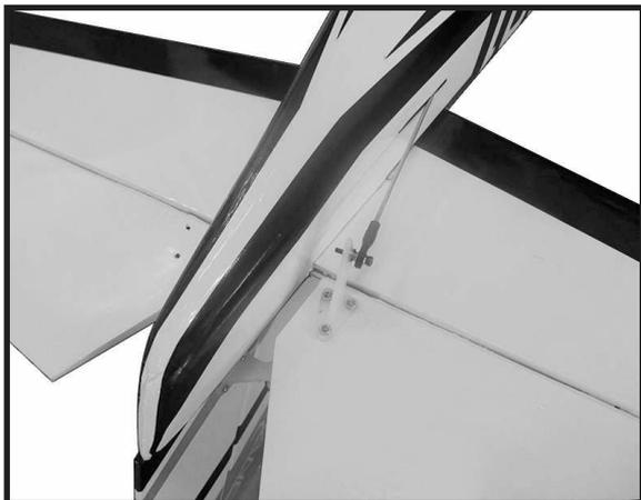
With the radio on and the elevator stick and trim centered, use a ruler to check that the elevator is aligned with the stabilizer.
