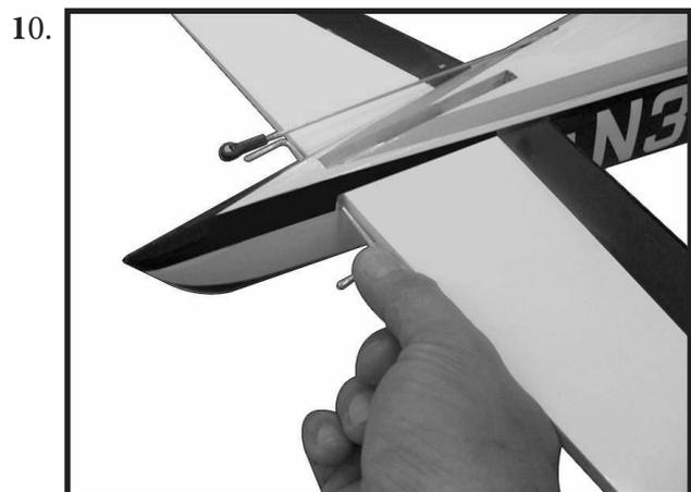
Slide the stabilizer partially into the fuselage so the wood at the center is exposed. Mix 1/2 ounce (15ml) of 30-minute epoxy. Use an epoxy brush to apply the epoxy to the exposed wood on the top of the stabilizer.
