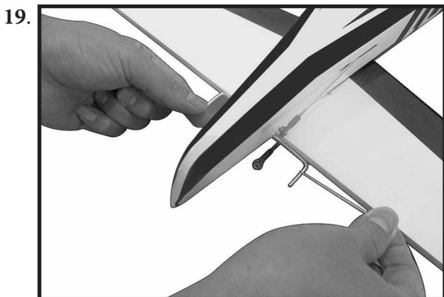
Use a toothpick to apply epoxy to the stabilizer where it contacts the joiner wire.
