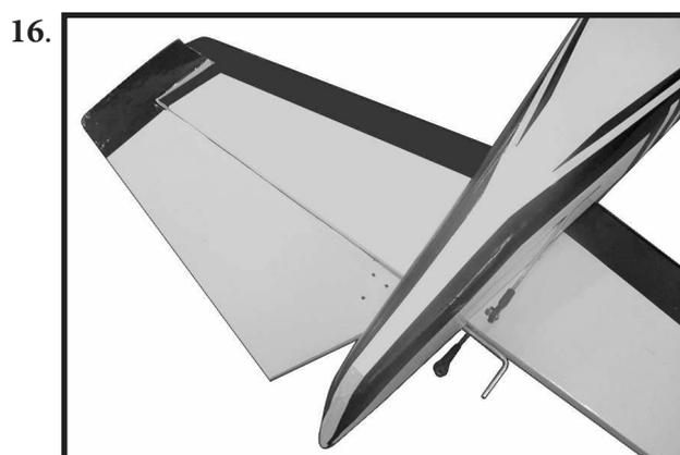
Check the fit of both elevators at this time. Once checked, remove the elevators.
