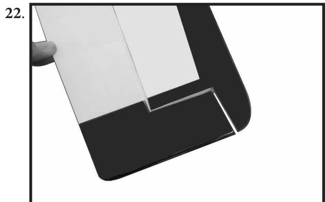
Flex the elevator slightly, making sure to keep the gap between the elevator and stabilizer as narrow as possible. Saturate each of the hinges using thin CA. Apply CA to the top of the hinges.
