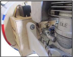
Attach throttle pushrod to the carburetor throttle arm with the ball link.
