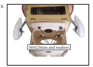
Attach the motor mount to the front of the electric motor box using four 4mm blind nut, four M4x25mm hex head bolts to secure the motor. Please see picture shown.
