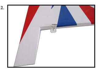
Slide the wing panel on the aileron until there is only a slight gap. The hinge is now centered on the wing panel and aileron. Remove the T-pins and snug the aileron against the wing panel. A gap of 1/64" or less should be maintained between the wing panel and aileron.
