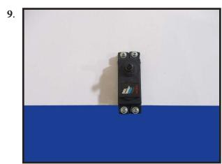
Tape the servo lead to the wing to prevent it from falling back into the wing.
