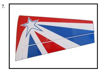
Note: Work the aileron up and down several times to "work in" the hinges and check for proper movement.
