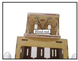
Attach the motor to the front of the electric motor box using four 4mm blind nut, four M4x20mm hex head bolts to secure the motor. Please see picture shown.
