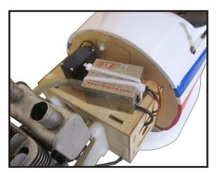
Connect ignition module to pickup line of engine. Secure with Safety Clip, safety wire, tape or other method. Ensure the plugs will not come apart from vibration or light tension.
