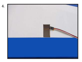
Attach servo lead to the aileron servo. Attach the string to the servo lead and carefully thread it though the wing. Once you have thread the lead throught the wing, remove the string so it can use for the other servo lead.
