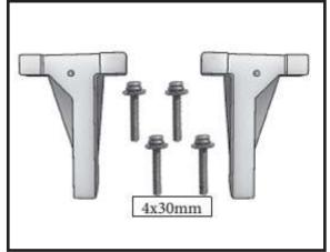
Use four 4x30mm head bolts and four 4mm washers to attach the engine mount rails to the fiewall. Tighten the screws . Make sure to use threadlock on the screws to help prevent them from vibrating loose.
