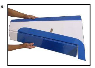
Turn the wing panel over and deflect the aileron in the opposite direction from the opposite side. Apply thin C/A glue to each hinge, making sure that the C/A penetrates into both the aileron and wing panel.
