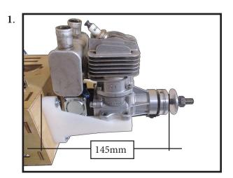
Use a pin drill and 4mm drill bit to drill a small indentation in the mount for the engine mounting screw.
