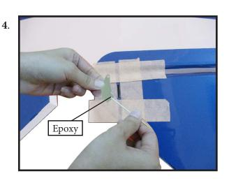
INSTALL ELEVATOR CONTROL HORN
