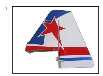
the top of the fuselage. The rear edge of the stabilizer should be flush with the rear edge of the fuselage and the lower rudder hinge should engage the precut hinge slot in the lower fuselage. The bottom edge of the stabilizer should also be firmly pushed against the top of the horizontal stabilizer.
