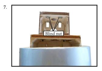
Attach the motor to the front of the electric motor box using four 4mm blind nut, four M4x20mm hex head bolts to secure the motor. Please see picture shown.
