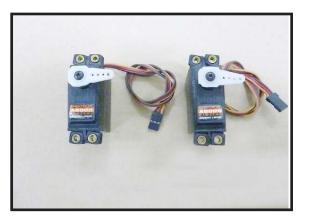
Minimum servo spec. Torque : 80 oz-in (5.8 kg-cm) @ 4.8V; 100 oz-in (7.2 kg-cm) @ 6.0V
