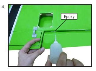
Turn the wing panel over and deflect the aileron in the opposite direction from the opposite side. Apply thin C/A glue to each hinge, making sure that the C/A penetrates into both the aileron and wing panel.
