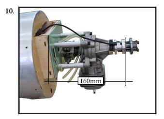
Position the engine with the drive washer (160mm) forward of the firewall.
