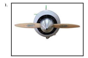
The propeller should not touch any part of the spinner cone. If it does, use a sharp modeling knife and carefully trim away the spinner cone where the propeller comes in contact with it.
