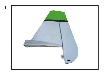
Using a modeling knife, remove the covering from over the precut hinge slot cut into the lower rear portion of the fuselage. Ths slot accepts the lower rudder hinge.
