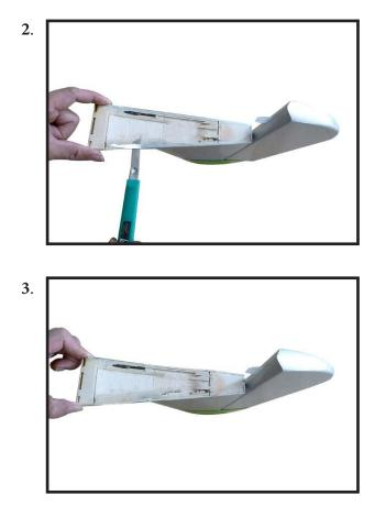
Slide the vertical stabilizer into the slot in the top of the fuselage. The rear edge of the stabilizer should be flsh with the rear edge of the fuselage and the lower rudder hinge should engage the precut hinge slot in the lower fuselage. The bottom edge of the stabilizer should also be fimly pushed against the top of the horizontal stabilizer.
