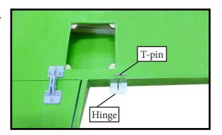
Slide the wing panel on the aileron until there is only a slight gap. The hinge is now centered on the wing panel and aileron. Remove the T-pins and snug the aileron against the wing panel. A gap of 1/64" or less should be maintained between the wing panel and aileron.
