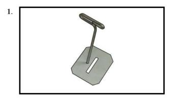
Remove each hinge from the wing panel and aileron and place a T-pin in the center of each hinge. Slide each hinge into the wing panel until the T-pin is snug against the wing panel. This will help ensure an equal amount of hinge is on either side of the hinge line when the aileron is mounted to the aileron.
