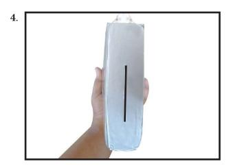
While holding the vertical stabilizer fimly in place, use a pen and draw a line on eachside of the vertical stabilizer where it meets the top of the fuselage.
