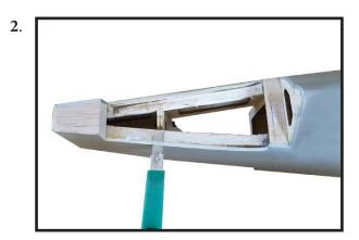
Slide the stabilizer into place in the precut slot in the rear of the fuselage. The stabilizer should be pushed firmly against the front of the slot.
