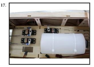
Reinstall the servo horn by sliding the connector over the pushrod wire. Center the throttle stick and trim and install the servo horn perpendiular to the servo center line. 18.
