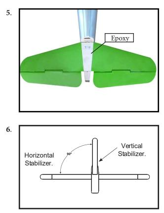
Slide the vertical stabilizer back inplace. Using a triangle, check to ensure that the vertical stabilizer is aligned 90° to the horizontal stabilizer.
