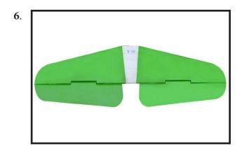
When you are sure that everything is aligned correctly, mix up a generous amount of 30 Minute Epoxy. Apply a thin layer to the top and bottom of the stabilizer mounting area and to the stabilizer mounting platform sides in the fuselage. Slide the stabilizer in place and realign. Double check all of your measurements once more before the epoxy cures. Hold the stabilizer in place with T-pins or masking tape and remove any excess epoxy using a paper towel and rubbing alcohol.
