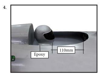
Epoxy canopy onto the fuselage. Trace around the canopy and onto the fuselage using a epoxy.
