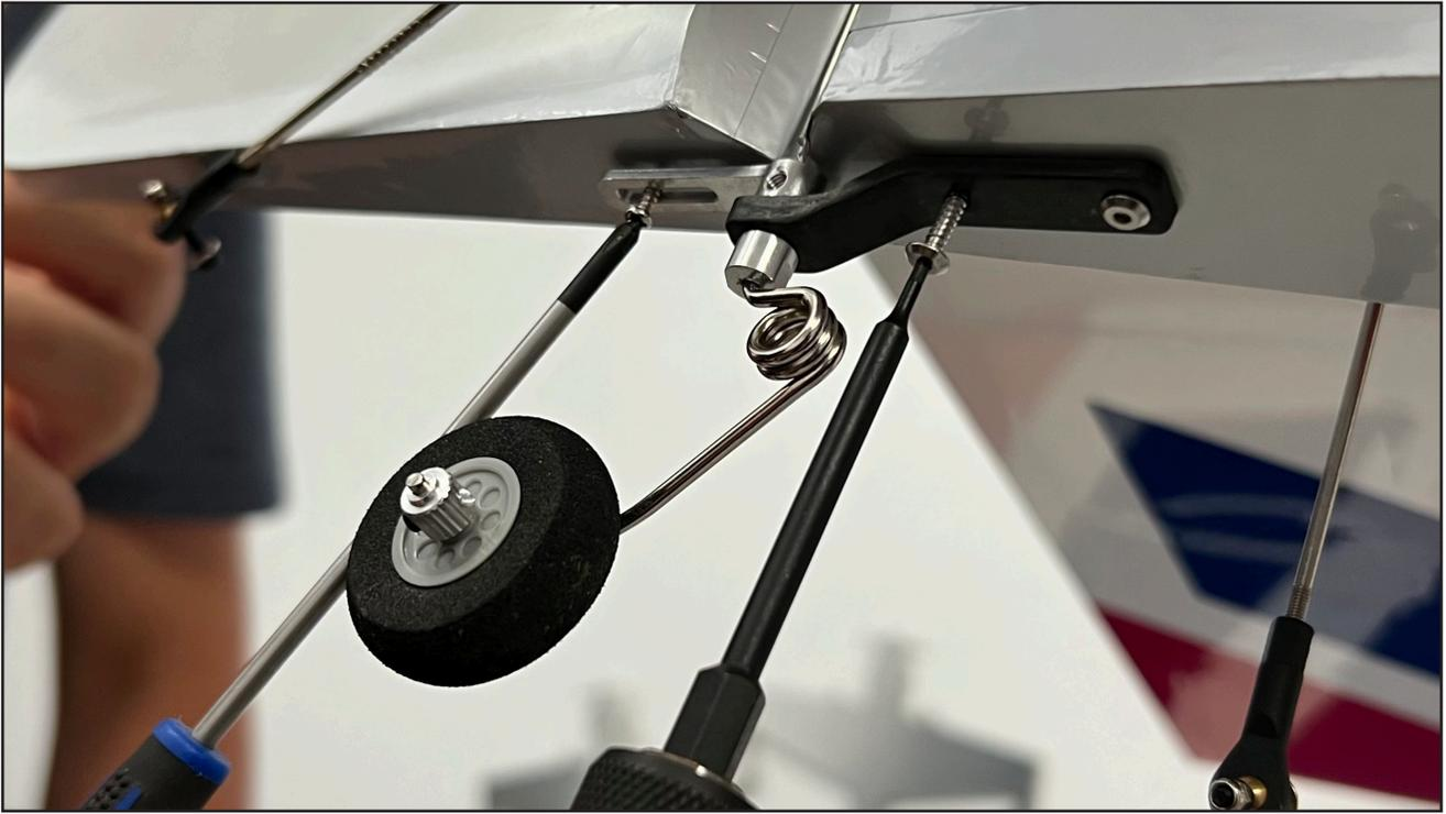
**8** Attach the rudder pushrod to the rudder servo arm as shown, tightening the locking nut on the back side of the servo arm.
