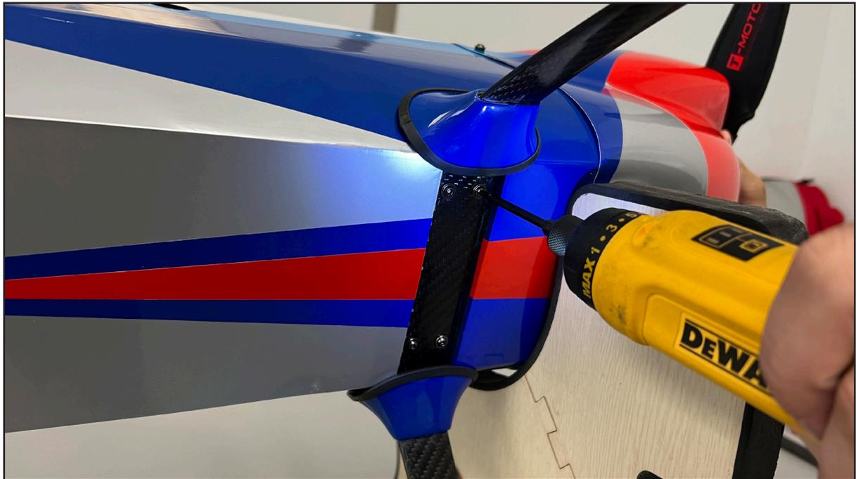
Attach the landing gear to the fuselage using screws, apply a drop of threadlocker to each screw.
