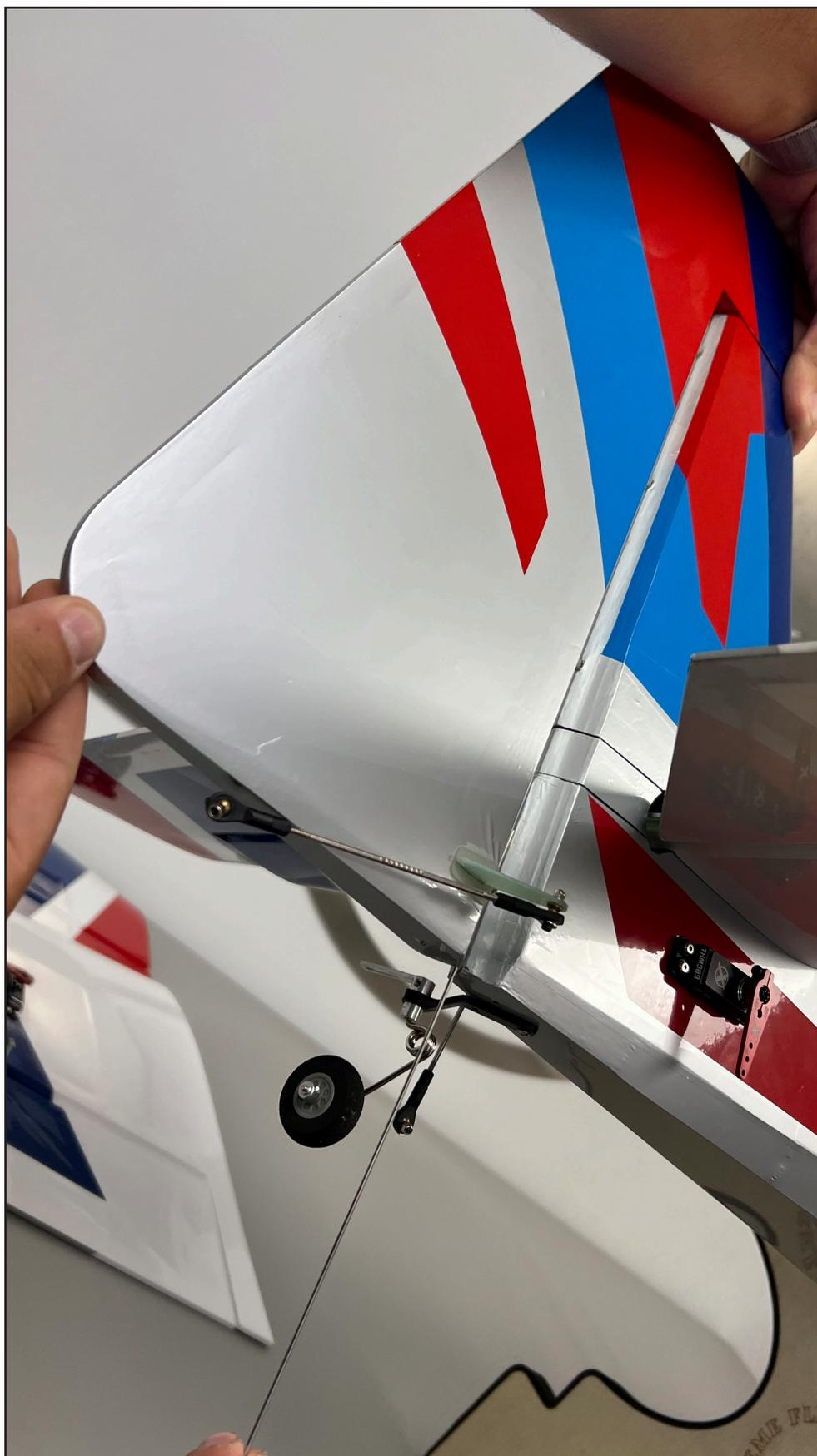
**7** Straighten and re-attach the tailwheel bracket and replace the screw. Add the tailwheel tiller screw into the bottom of the rudder as shown. Make sure the tailwheel and rudder move freely together.
