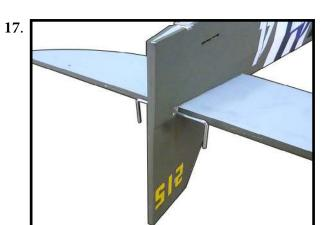
Mix a small amount of 15-minute epoxy. Use a toothpick to apply epoxy to the joiner wire.
