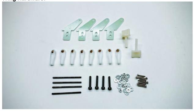
1. Locate the 2 wing panels as well as the composite aileron and flap control horns. Use sandpaper to scuff the portion of the control horn that will be glued into the surface. For a more finished look you may wish to paint your control horns before installation. We used a black Sharpie to perform this task with great results. Do not paint the portion of the control horn that will glue into the control surface!
