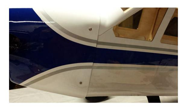
70. Use a sharp hobby knife or soldering iron to remove the covering over the air escape holes in the bottom of the
