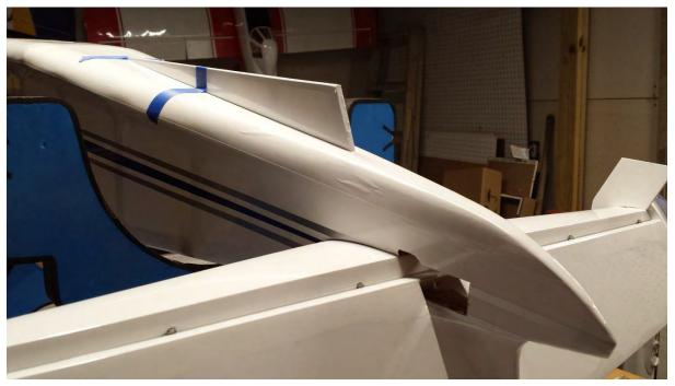
33. Attach an 18" servo extension to your elevator servo and using the manufacturer supplied hardware install it with the output shaft towards the rear of the fuselage. Assemble the pushrod and install as shown in the picture.
