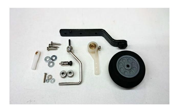
35. Attach the wheel to the Axle with the supplied wheel collar. NOTE: It is a good idea to file a small flat section on the axle for the wheel collar set screw to mate up to.
