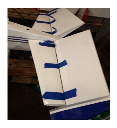
29. Locate the fences for the horizontal stab and attach them with medium CA. Make sure to confirm alignment with the vertical stab.
