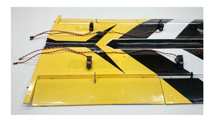
13. Use the manufacturer supplied mounting hardware to install the servos with the output shaft toward the LEADING EDGE of the wing. Electronically center the servo and install 1.25" servo arms onto the servo spline. The servo arms should be parallel to the hinge line when centered. *It is very important that you use the same length servo arms for both flap and aileron servos*.
