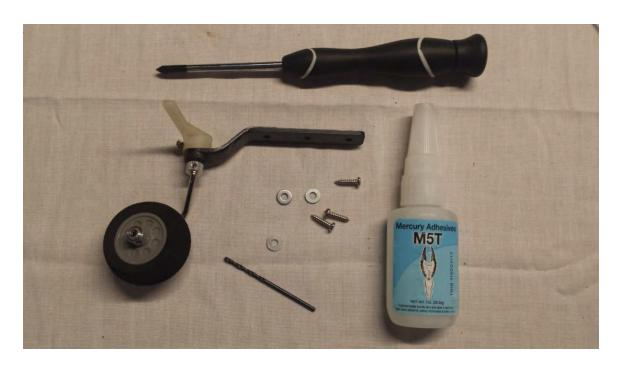
37. Locate the Tailwheel pushrod (29.5" and threaded on one side) and insert it through the hole on the pilot's upper left side and into the guide tube, threaded end first.
