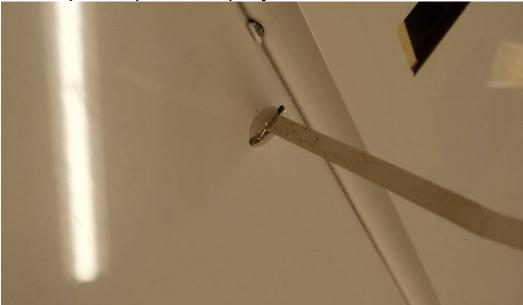
5. Install the control horns into their respective slots and wipe away any excess epoxy with a paper towel or cloth soaked with denatured alcohol.
