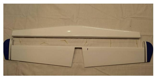
24. Insert the elevator section Upside-down and backwards into the Stab/Elevator slot
