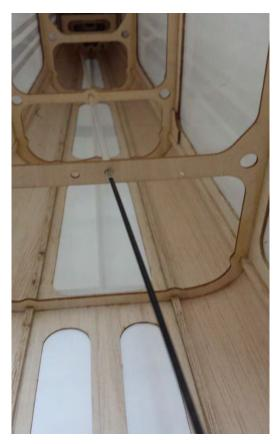
38. Push the control rod carefully until you feel resistance, locate the area where the control rod is trying to poke thru the covering and use a sharp hobby knife or soldering iron to remove the covering from this location. It is easiest to do this with the fuselage upside down in a stand.
