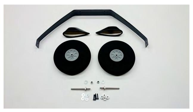
20. Attach the landing gear to the fuselage using the supplied bolts and washers. The landing gear has a slight airfoil, make sure that the thicker part of the gear is facing the nose of the airframe.
