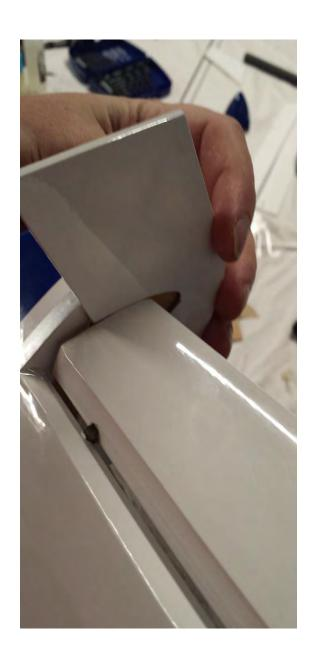
30. Locate the lower keel. Note that the small extension piece (top piece in picture) is to be used when building the airframe for float flying only as it will occupy the space for the tailwheel.
