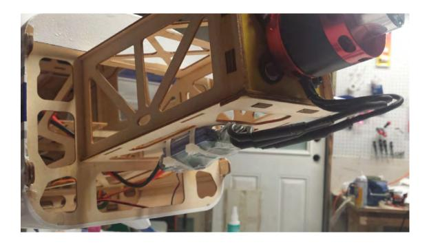
63. Attach a 12" servo wire extension and a 8-10" battery extension to the ESC and route them into the fuselage. There are
