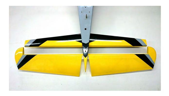
26. Check that the horizontal stabilizer is centered and properly aligned with the main wings. It is a good idea to use a tape measure and triple check all measurements before gluing the Stabilizer in place. Measure from a fixed point on the wings to the tip of the Stabilizer on both sides. Adjust the stab until both sides are the same. Take your time with this step as proper alignment is critical.
