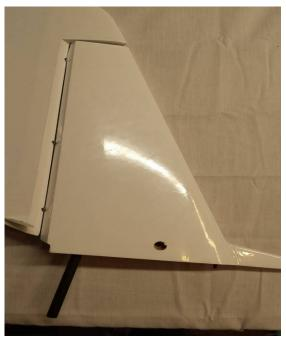
44. Slide the completed assembly into the vertical stab tube socket and secure the stab to the fuselage with a 4mm cap head screw. Don't forget to use thread lock!
