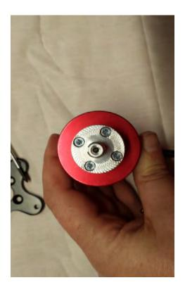
56. Secure the prop adapter to the motor with supplied socket head cap bolts using blue thread lock on each bolt.
