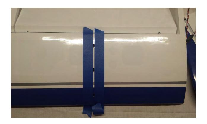
17. Use 30 min epoxy to attach the fences. Wipe away any excess epoxy with a paper towel soaked in acetone. Be sure to remove the tape before the epoxy fully cures. Repeat this process for the other wing panel.
