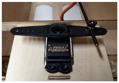
49. Next install the pull-pull cables and ball links. It is easiest to build the rear half (rudder side) of the cables and install them
