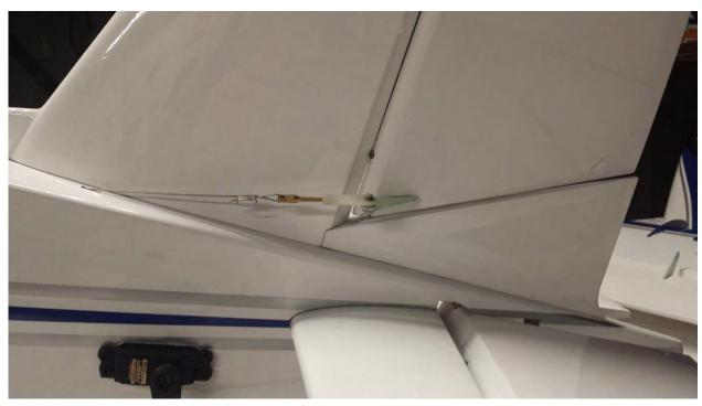
50. Follow this same method to assemble the linkages in the forward part of the system that will attach to the servo arm. The cables should cross in the fuselage for proper function. Adjust
