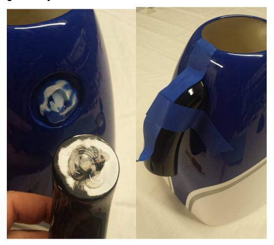
67. When the glue for the exhaust stacks is fully cured, tear 4 short pieces of painter's tape and place each piece of tape on the side of the fuselage so that each piece corresponds with one of the 4 cowl mounting tabs. Use a felt tipped pen to mark the location of the center of each mounting tab.
