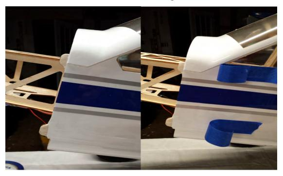
68. Slide the Cowl into position. Install the spinner onto the motor shaft for reference and once satisfied with the cowl position, roll the tape back into place and secure the cowl. Use a 1/16" drill bit to drill a hole at the location of the dot on each piece of tape.
