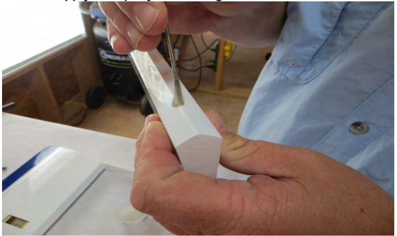
9. Apply epoxy to the barbed section of the hinge on one side and insert it into the hole until the center of the hinge is centered on the hinge line. Using a paper towel soaked with acetone or denatured alcohol wipe away any epoxy that has been squeezed out of the hole.
