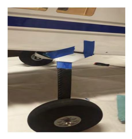
22. Locate the 2 axles, 2 locking nuts, 2 wheels, 4 wheel collars and 2 washers and mount the wheels as shown.
