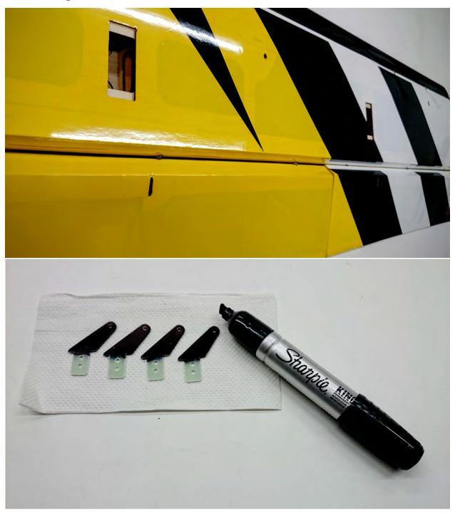
2. Using a soldering iron or a SHARP hobby knife, remove the covering from the slots for the aileron and flap horns.
