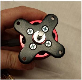
59. Locate the 4mm black cap bolts and washers to attach the assembled motor to the firewall.
