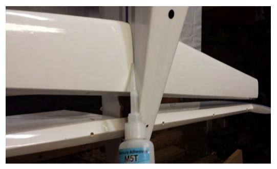
28. Once the horizontal stab is glued in place, use the same technique to install the elevator hinges and control horn that we used for the aileron and flaps.
