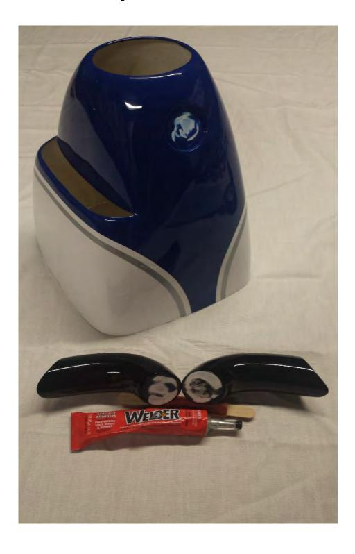
66. Using contact adhesive or epoxy glue the exhaust stacks to the cowling and hold them in place with painter's tape until the glue is dry.
