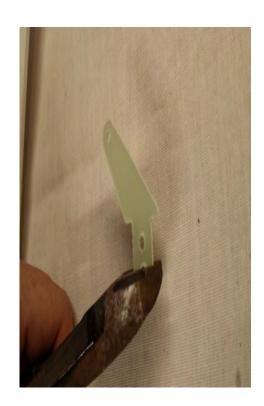
42. When satisfied with the fit of the control horns, mix up a small batch of epoxy and install the rudder control horns.
