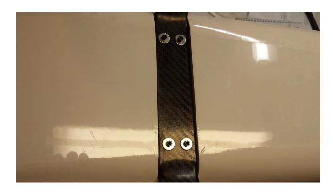
21. Slide the gear fairings into place against the bottom of the fuselage. Use a piece of painters to mark their location. Remove the fairing and apply a thick bead of Goop to the carbon gear just above the tape line. Slide the fairing back into place and secure with tape until dry.
