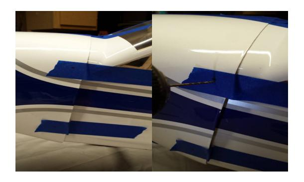
69. Remove the tape and cowl and add a drop of CA to each hole. Mount the cowl with the 4 of the small wood screws included with the kit.
