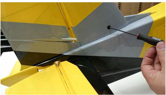
45. Deflect the rudder to one side and install the vertical stab wedge. Wick in a bit of CA to hold it in place.
