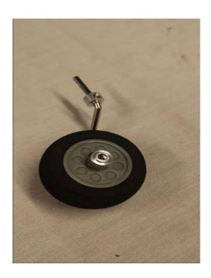
36. Next install the carbon fiber mounting bracket and tiller arm. Make sure to align the screw in the tiller arm with the flat spot on the tailwheel shaft and use thread lock!
