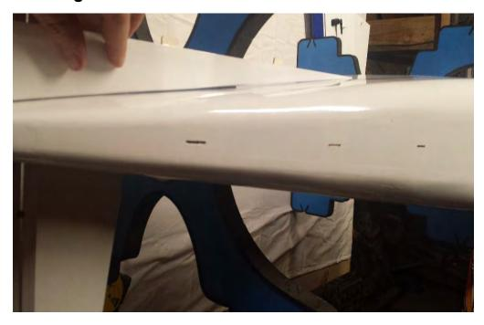
32. Dry fit the lower keel in position and when happy with the fit, use 30-minute epoxy to attach it to the fuselage. Use tape to secure while drying. Be sure to check for proper alignment!
