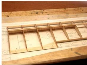
58...Glue the 3/32" sq. stringer spars into position. They should stop at W-9.
