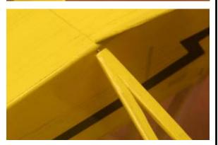
112...Place 1/2" pieces of aluminum tube over the wires at the outboard ends of the wing struts. Place the ends of the struts on the bottom of the wing over the W-21's. Adjust the bends on each end of the struts so the tubes lay flat on the bottom of the wing. Mark the location of the tubes on the wing. Remove the struts and glue the tubes to the bottom of the wing. Reinstall the struts to check the fit.
