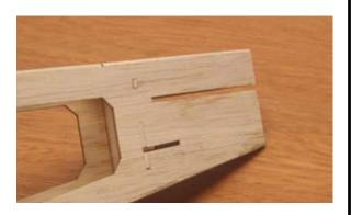
30...Test fit the tail surfaces on the fuselage. Trim and sand if needed to achieve the proper fit. Cut the bottom rudder hinge slot in the end of the fuselage.
