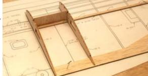
53...Glue ribs W-4 thru W-9 into position. They should be 90 degrees to the building board. Do not glue W-9 to W-18 at this time.
