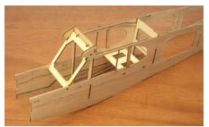
8...Place part F-10 into position in the fuselage but do not glue at this time. Glue the firewall (F-11) into position making sure the front of the fuselage is not twisted. Now glue F-10 into position.
