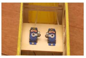
94...Install the pushrods into the housings. Secure the rear of the pushrods with Mini E/Z Links.
