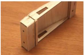
42...Slide the short end of the two joiners into the slots in the W-1 ribs. The outboard ends of the joiners should angle up. The inboard ends should meet at the centerline on W-12. Glue the joiners to W-12 and the top and bottom spar.
