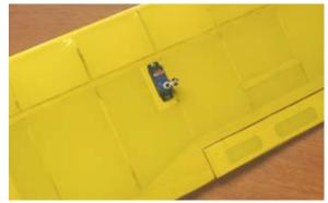
106...Glue the aileron control horns into position on the bottom of the ailerons. Drill 1/16" holes for the pins to fit into.
