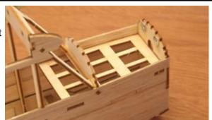
21...Using the 3/32" sq. X 18" strips, glue the stringers to the top front fuselage between F-11 and F-21. Trim the stringers flush with the formers.
