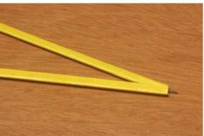
110...Drill a 1/16" hole in the fuselage sides and carefully glue a 1/2" piece of the aluminum tube in place, flush with the fuselage side.
