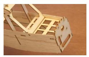
9...Place F-12 into position. The blind nuts are a little closer to the front edge. Glue securely into position.
