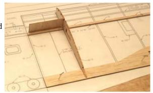
52...Glue rib W-2 into position. The top of the rib should angle slightly toward the wing tip.
