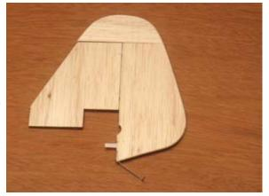
2...Sand the 1/8"x 3" dowel to 3/32" diameter. Join the elevators (S-2) using this dowel. Use the stabilizer as a guide. Trim the dowel if required to achieve the proper length.
