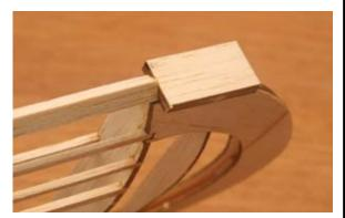
68...Glue the aileron servo tray (W-20) into position on rib W-5. Glue to the rib as well as the main spar. The front edge should be flush with the spar.
