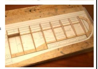
54...Pin the W-10 rib into position on the plan. The standoffs should be placed on the hatched areas on the plan.
