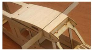
47...Place the W-15 discs onto the nylon screws and thread them into place. Glue the W-15's to the top of the center section.
