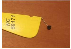
91...Attach the rudder with the hinges and glue in place.
