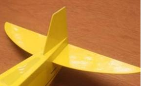
89...Attach the elevators with the hinges and glue in place.
