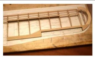
61...Roll the front of the wing tip forward and glue to W-9 and W-10. The very end of the wing tip should be level with (the same height) as the main spar at rib W-9.
