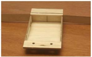
43...Center W-12A on the back of the joiners and glue into position.
