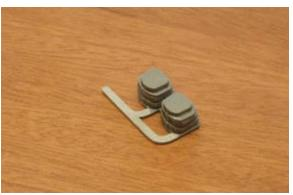
117...Glue the 3/8" blocks to the front of F-11. They should be flush with the outside of the fuselage. Trim the top block to provide clearance for the motor.
