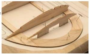
55...Glue the 3/32" x 3/16" top spar into position. The spar stops at the W-9 rib. Glue the 1/4" sq. leading edge into position in the notches in the front of the ribs. The leading edge stops at rib W-9. Be careful to not allow glue to run down onto W-18.
