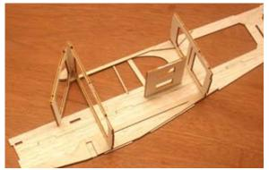
7...Place the left fuselage side into position and square up the fuselage. Glue the left fuselage to the formers. Make sure that the fuselage is square and completely glue the formers to the fuselage sides.
