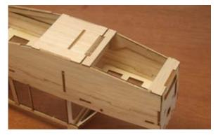
15...Place former F-17 into position and pull the rear of the fuselage sides together. Adjust the back end until the fuselage is straight and square. Glue the fuselage sides together and glue the former in place.
