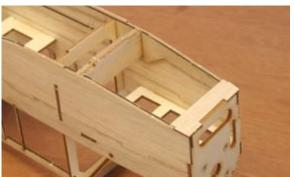
14...Glue F-15 and F-16 into position on the bottom of the fuselage.
