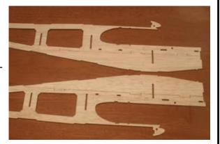
4...Glue the F-2 and F-3 doubelers to the inside of the F-1R & F-1L fuselage sides. Be sure to make a right hand and a left hand side.
