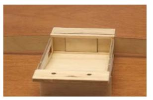
44...Sheet the bottom of the center section with the 1/16" sheet as you did the top.
