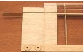
84...Slide the wing joiner on the center section into position in the left wing. Position it tightly between the spars and forward against the shear web and glue the left wing to the center section.
