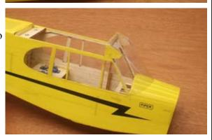
96...Insert the landing gear wire into the slot in the fuselage. Make sure it is completely seated. Squirt two drops of thin C/A into the slot and let dry completely.
