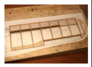
59...Glue the top trailing edge / wing tip parts W-16, W-17 and W-18T together.
