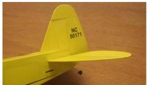
92...Glue the rudder and elevator control horns into position. Drill 1/16" holes for the pins to pass thru. When the glue is dry, cut off the excess pins flush.
