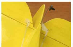
The front ends of the pushrods are attached to the servos with Mini E/Z Connectors. Glue the pushrod housings to the former.
