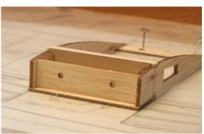
38...Glue the second W-14A into position on the front of the previous one. Now glue W-14B into position on front of the W-14A's.
