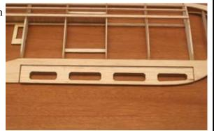
82...Cut slots in both W-1 ribs at the dashed lines to accept the wing joiner as shown on the plan.
