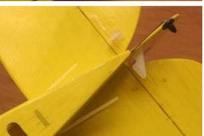
The front ends should pass thru the slot in former F-7. Glue the housings to the rear exits. Do not glue the front ends to the former at this time.
