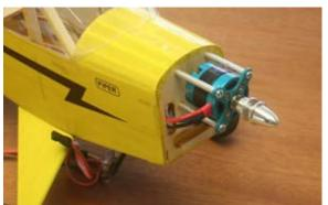
101...Secure the speed controller to the fuselage with velcro. Plug the motor into the speed controller.
