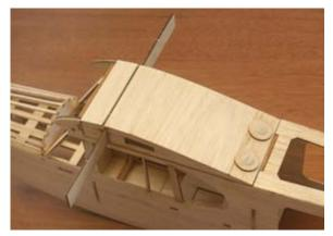
48...Glue W-23 into position on the sheet on the bottom of the center section. Cut away the sheet from the center when the glue dries.
