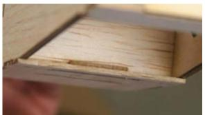
27...Test fit the hatch to the bottom of the fuselage. The front tab (H-2) slides under part F-13. Slide the hatch slider forward and press the back end of the hatch down on the fuselage. Move the slider back to secure the hatch. Trim the 1/16" spacer as required to allow the slider to move to the rear. You can trim the outside edges of H-2 to center the front of the hatch if required.
