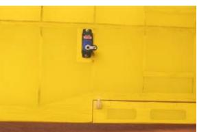
107...Install the pushrods. Attach the rear of the pushrods to the horns with Mini E/Z Links. The front ends are attached to the servos with Mini E/Z Connectors. When the servos are in neutral the servo arm should be 30 degrees forward as shown.
