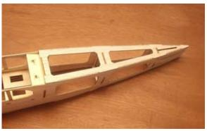
19...Glue F-20 into position on the bottom of the fuselage.
