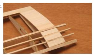
71...Trim the spars, leading edge and trailing edge flush with the end of the wing.
