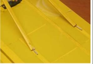
113...Glue two 1" long pieces of 3/32" sq. balsa into the holes in M-1. They should be 90 degrees to M-1.
