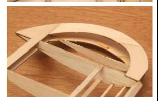
63...Cut part way thru the bottom of W-16 at the outside edge of W-9.
