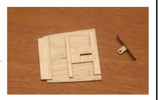
24...Place parts H-7 into position on the hatch. Insert H-5/6 into position to establish the proper spacing for the H-7's. Use the tip of a straight pin to apply a tiny amount of glue to the outside edges of the H-7's. Use extreme care to make sure that you DO NOT glue the H-5/6 slider into position!!!
