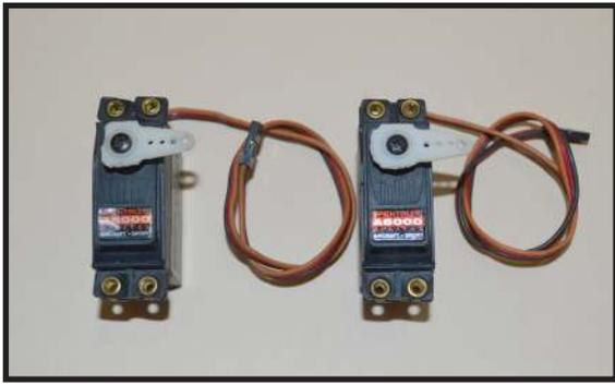
⚠ Because the size of servos differ, you may need to adjust the size of the precut opening in the mount. The notch in the sides of the mount allow the servo lead to pass through.
