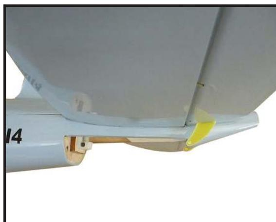
3) Thread one clevis and M2 lock nut on to each elevator control rod. Thread the horns on until they are flush with the ends of the control rods.
