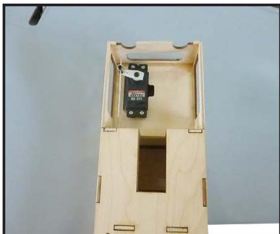
4) Move the throttle stick to the closed position and move the carburetor to closed. Use a 2.5mm hex wrench to tighten the screw that secures the throttle pushrod wire. Make sure to use threadlock on the screw so it does not vibrate loose.
