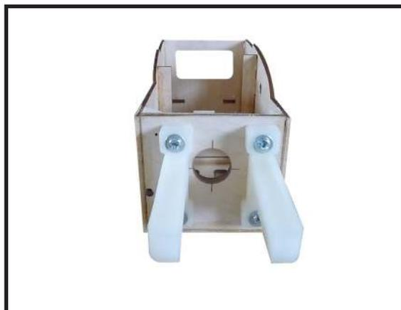
1) Position the engine with the drive washe (118mm) forward of the firewall as shown.
