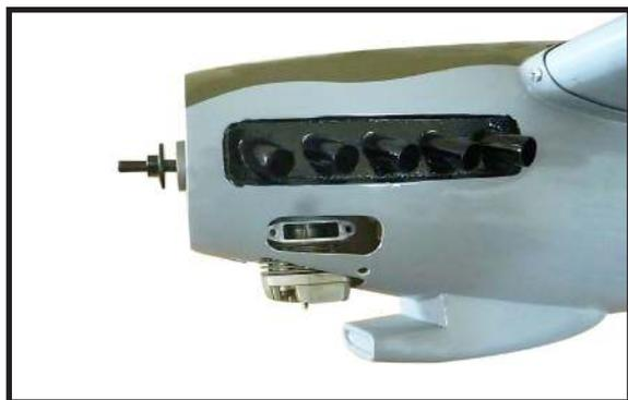
3) Install the muffler and muffler extension onto the engine and make the cutout in the cowl for muffler clearance. Connect the fuel and pressure lines to the carburetor, muffler and fuel filler valve. Secure the cowl to fuselage using the M3x10mm screws.
