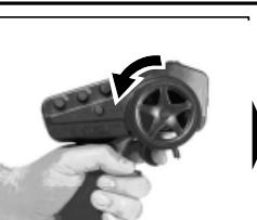
Go to full left on the transmitter and back to neutral. Orange light will go off when moving the steering wheel and go back to solid when accepted.
