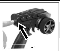
Whilst holding the bind button on the transmitter press the ON button. Wait until the orange light on the receiver goes solid.
