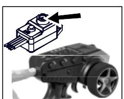
Turn off the ESC and then turn off the transmitter. Binding is complete.
