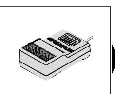
The Orange light on receiver will flash rapidly, you can remove your finger from the receiver bind button when this happens.
