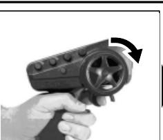
Go to full right on the transmitter and back to neutral. Orange light will go off when moving the steering wheel and go back to solid when accepted.
