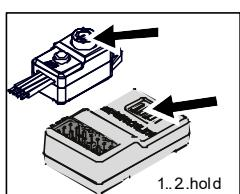
Press the ESC power button and quickly press the bind button on the receiver 3 times. On the third press keep holding the bind button.
