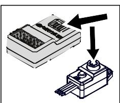
Press and hold bind button on the receiver then press the power button on the ESC. Orange light on receiver will flash rapidly.
