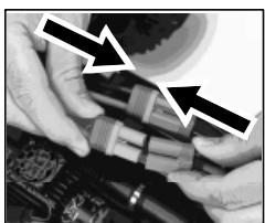
Connect a fully charged battery pack to the ESC.
