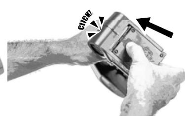
**CAUTION:** Only charge rechargeable batteries. Charging non-rechargeable batteries may cause the batteries to burst, resulting in injury to persons and/or damage to property.
