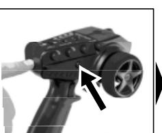
Whilst holding the bind button on the transmitter press the ON button. Wait until the orange light on the receiver goes solid.
