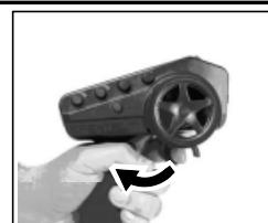
Go to full throttle on the transmitter and back to neutral. Orange light will go off when moving the trigger and go back to solid when accepted.
