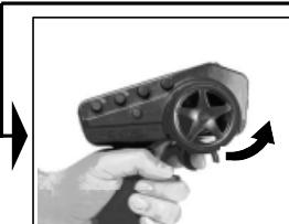
Go to full brake on the transmitter and back to neutral. Orange light will go off when moving the trigger and go back to solid when accepted.
