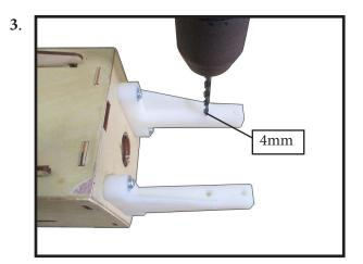
The fire wall has the location for the throttle pushrod tube (pre-drill).
