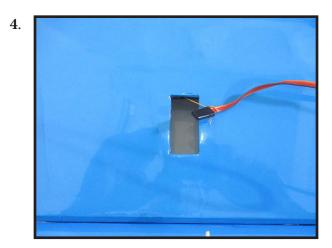
Attach servo lead to the aileron servo. Attach the string to the servo lead and carefully thread it though the wing. Once you have thread the lead throught the wing, remove the string so it can use for the other servo lead.
