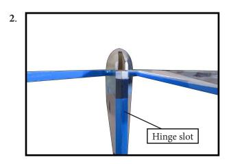
Slide the vertical stabilizer into the slot in the top of the fuselage. The rear edge of the stabilizer should be flush with the rear edge of the fuselage and the lower rudder hinge should engage the precut hinge slot in the lower fuselage. The bottom edge of the stabilizer should also be firmly pushed against the top of the horizontal stabilizer.
