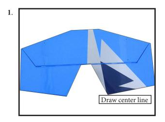
Using a modeling knife, carefully remove the covering at mounting slot of horizontal stabilizer ( both side of fuselage).
