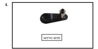
Reinstall the servo horn by sliding the connector over the pushrod wire. Center the throttle stick and trim and install the servo horn perpendicular to the servo center line.
