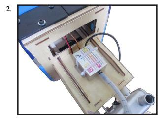
Connect ignition module to pickup line of engine. Secure with Safety Clip, safety wire, tape or other method. Ensure the plugs will not come apart from vibration or light tension.
