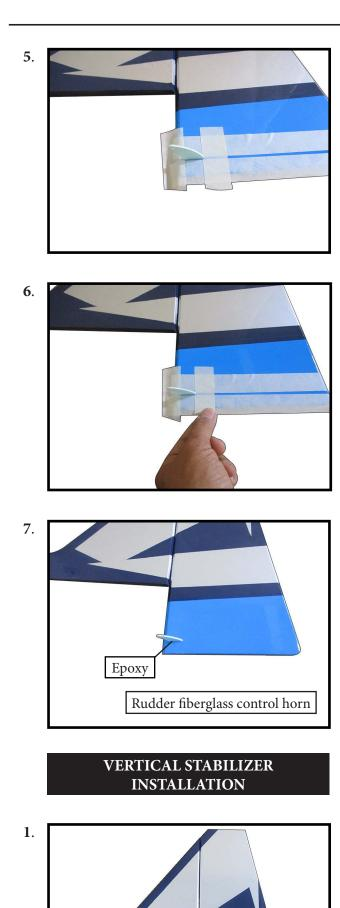
Using a modeling knife, remove the covering from over the precut hinge slot cut into the lower rear portion of the fuselage. This slot accepts the lower rudder hinge.
