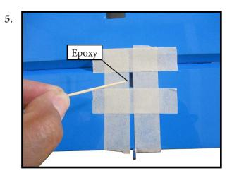
Apply epoxy to the area of the control horns that fist into the slots. Use enough epoxy so the control horns will be fully bonded to the fied surfaces.
