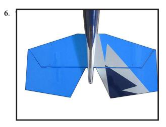
After the epoxy has fully cured, remove the masking tape or T-pins used to hold the stabilizer in place. Carefully inspect the glue joints. Use more epoxy to fill in any gaps that may exist that were not filled previously and clean up the excess using a paper towel and rubbing alcohol.
