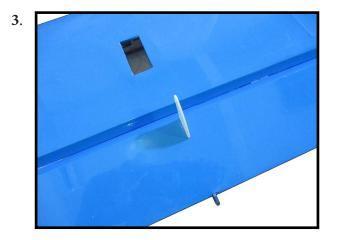
Place low-tack tape 1/32 inch (1mm) from the control horn slot. This will prevent epoxy from getting on the control surface when the control horns are glued in place.
