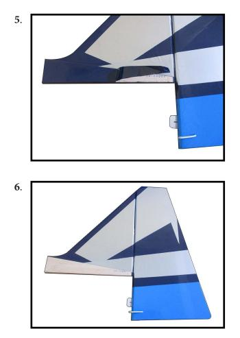
Slide the vertical stabilizer back inplace. Using a triangle, check to ensure that the vertical stabilizer is aligned 90° to the horizontal stabilizer.
