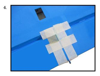
Remove the control horns from the control surfaces. Apply epoxy to the slot in the aileron and flap. Make sure the epoxy gets into the slot for a good bond between the surfaces and control horn.
