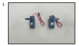
Maximum Servo spec. Torque : 126.6 oz-in (9.11 kg-cm) @ 6.0V; 178 oz-in (12.82 kg-cm) @ 7.4V; 248 ozin (17.86 kg-cm) @ 8.4V
