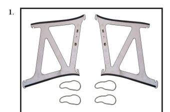
Locate the wing transport frames and rubber bands. Slide the frames between the top and bottom wing as shown. Use a rubber band to hold the frame to the top and bottom wing.
