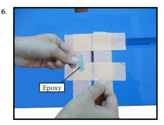
Before the epoxy fully cures, remove the tape from around the control horn. This will allow the epoxy to flow around the control horn, creating a small filet between the control horn and surface for a filshed look and secure bond.
