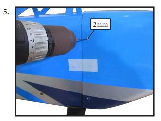
Install the muffler and muffler extension onto the engine and make the cutout in the cowl for muffler clearance. Connect the fuel and pressure lines to the carburetor, muffler and fuel filer valve. Secure the cowl to fuselage using the M3x10mm socket head screws.Putting a small length of silicon fuel tube under the head of the screw helps with vibration.
