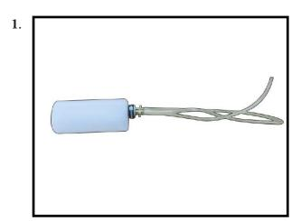
You should mark which tube is the vent and which is the fuel pickup when you attach fuel tubing to the tubes in the stopper. Once the tank is installed inside the fuselage, it may be difficult to determine which is which. Slide the fuel tank into the fuselage. Guide the lines from the tank through the hole in the fiewall.
