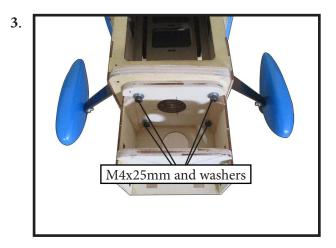
Attach the motor mount to the front of the electric motor box using four 5.5mm blind nut, four M4x25mm hex head bolts to secure the motor. Please see picture shown.
