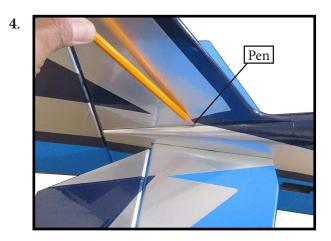
Remove the stabilizer. Using a modeling knife, remove the covering from below the lines you drew. Also remove the covering from the bottom edge of the stabilizer and the bottom and top edges of the filler block. Leave the covering in place on the sides of the filler block.
