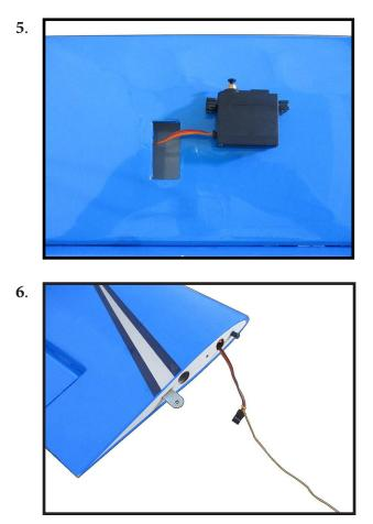
Tape the servo lead to the wing to prevent it from falling back into the wing.
