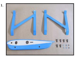
Remove the covering in the top of the fuselage for the cabane struts.
