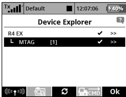
MTAG connected to the receiver Ext. port (EX Bus mode).
