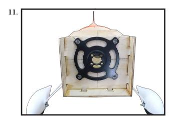
Then, use 8mm drill bit to enlarge the holes on the electric motor box.
