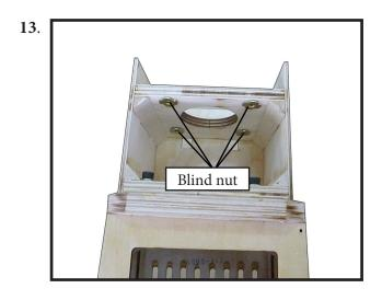
Attach the motor mount to the front of the electric motor box using four 4mm blind nut, four M6x25mm hex head bolts to secure the motor. Please see picture shown.
