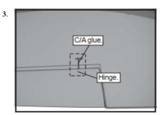
Deflect the aileron and completely saturate each hinge with thin C/A glue. The ailerons front surface should lightly contact the wing during this procedure. Ideally, when the hinges are glued in place, a 1/64" gap or less will be maintained throughout the lengh of the aileron to the wing panel hinge line.
