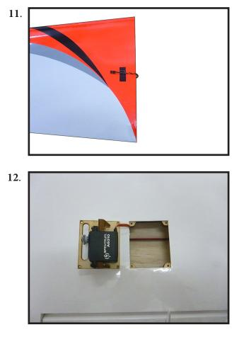
Set the aileron hatch in place and use a Phillips screw driver to install it with four wood screws.
