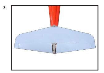
With the stabilizer held firmly in place, use a pen and draw lines onto the stabilizer where it and the fuselage sides meet. Do this on both the right and left sides and top and bottom of the stabilizer.
