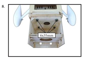
Attach the motor to the front of the electric motor box using four 4mm blind nut, four M6x35mm hex head bolts to secure the motor. Please see picture shown.
