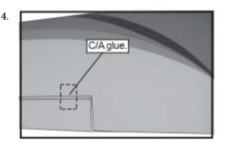
Turn the wing panel over and deflect the aileron in the opposite direction from the opposite side. Apply thin C/A glue to each hinge, making sure that the C/A penetrates into both the aileron and wing panel.
