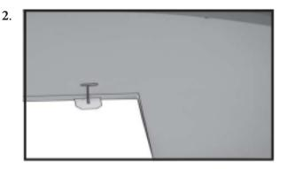
Slide the wing panel on the aileron until there is only a slight gap. The hinge is now centered on the wing panel and aileron. Remove the T-pins and snug the aileron against the wing panel. A gap of 1/64" or less should be maintained between the wing panel and aileron.
