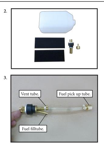
Carefully bend the second nylon tube up at a 45° angle. This tube is the vent tube.
