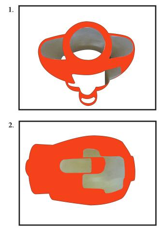
Tape the cowl to the fuselage using low-tack tape.
