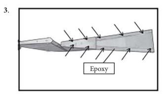
Slide the vertical stabilizer into the slot in the top of the fuselage. The rear edge of the stabilizer should be flush with the rear edge of the fuselage and the lower rudder hinge should engage the precut hinge slot in the lower fuselage. The bottom edge of the stabilizer should also be firmly pushed against the top of the horizontal stabilizer.
