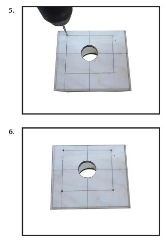
Attach the electric motor box to the firewall centered with the cross lines drawn on the electric motor box and firewall. Using M6x25mm to secure the motor box to the firewall. Please see pictures below.
