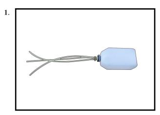
You should mark which tube is the vent and which is the fuel pickup when you attach fuel tubing to the tubes in the stopper. Once the tank is installed inside the fuselage, it may be difficult to determine which is which.
