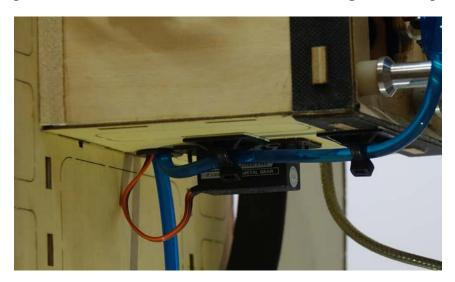
24. If using an electric motor we recommend mounting the ESC to the bottom of the motorbox either with screws, nylon cable ties or Velcro straps.
