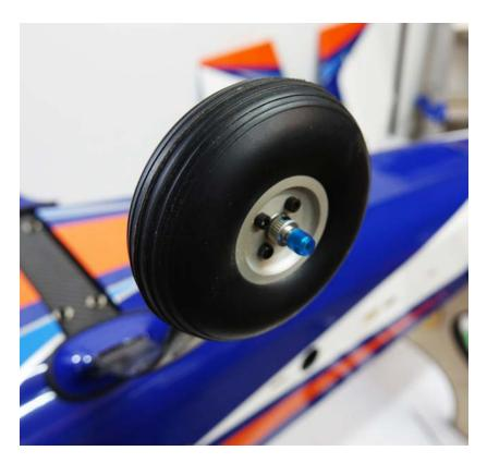
17. Reinstall the wheel pants and secure with 2 3mm bolts inserted through the carbon gear and into the blind nuts in the wheel pants. Be sure to use thread lock on the bolts! Tighten the setscrew to secure the wheel pant bracket to the axle.
