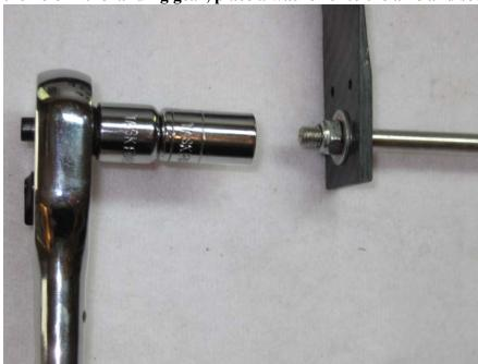
15. There is a pre-cut slot in the wheel pant to allow it to fit over the axle. You may need to open this slot with a rotary tool to allow it to slide into position over the axle. Screw the machined aluminum outer wheel pant bracket to the plywood spacers and secure to the interior wall of the wheel pant with epoxy, making sure it fits over the end of the axle and positions the wheel pant correctly.
