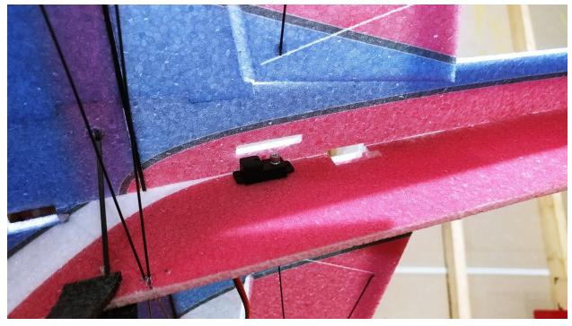
This is the location for the elevator servo. It will be placed between the aileron and rudder servo and on the underside of the fuselage. The servo arm will be pointed up as the control horn will be placed on the top of the elevator.
