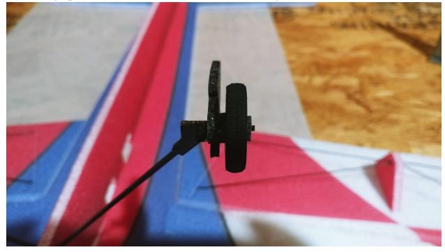
Next, slide on the smaller piece of foam that will act as the collar on the outside of the wheel. Once again, do not add any glue to this piece.
