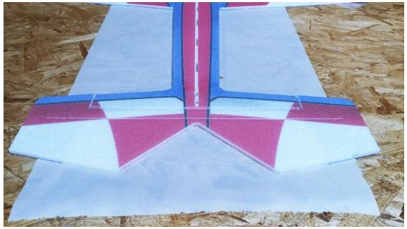
Test fit the horizontal stab/elevator into the rear of the fuselage. If all is well, glue into place making sure that it is flush with the fuselage and flat with the rest of the airplane.
