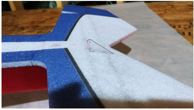
The elevator control horn is the shortest and will be placed as shown above. You will notice a small square shaped cutout on the underside. This is meant to be placed around the spar of the elevator that was installed earlier.
