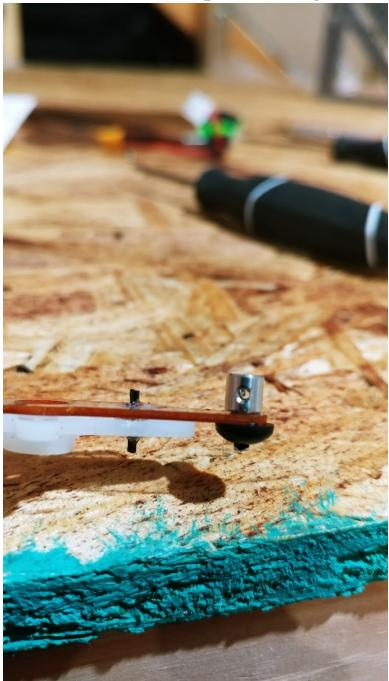
The mini EZ connector as shown above will be used to connect the linkage to the servo arm. It will be easiest to place these on the arm while it is off of the servo. Put the top piece through the hole in the arm, then fully clamp the bottom piece around the pin. The flat side of the bottom piece will be pushed against the servo arm. Leave the top screw loose for now until the control linkage is slid through.
