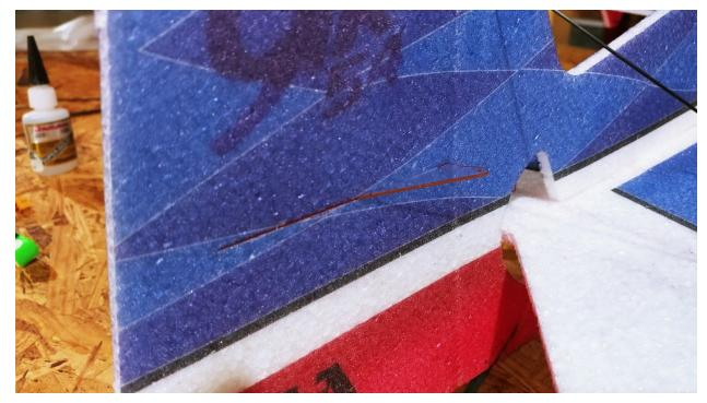
Locate the final control horn needed for assembly. The rudder uses the same type of control horn as the aileron which is on of the longer of the 4. If necessary, scuff the sides with sandpaper, test fit making sure the hole is directly above the hinge line, then glue in place. Make sure glue is used along the entirety of the control horn.
