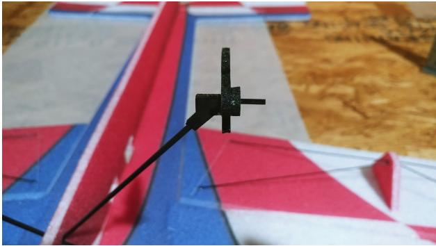
Next will be sliding on the larger foam collar. Add just a small amount of glue to hold this into place against the wheel spat.
