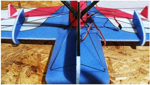
Shown is the configuration for the underside bracing of the "cowling" area. The two most forward pieces are 80mm, and the pieces that extend to the landing gear are 145mm.
