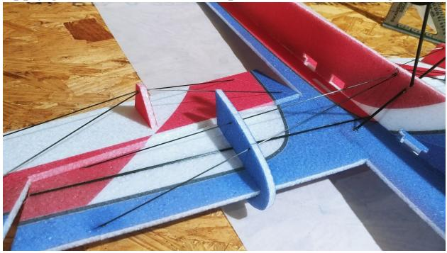
This is the configuration for the wing bracing. In total, there are 2 pieces of carbon fiber used per wing to accomplish this.
