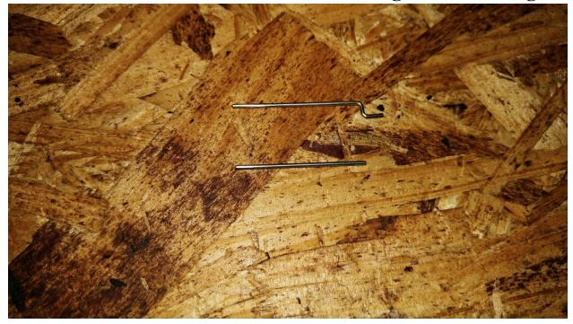
Above are what will be used for each end of the control linkages. The Z bend will be inserted into the control horn while the straight end will be slid into the opening of the mini EZ connector on the servo arm.
