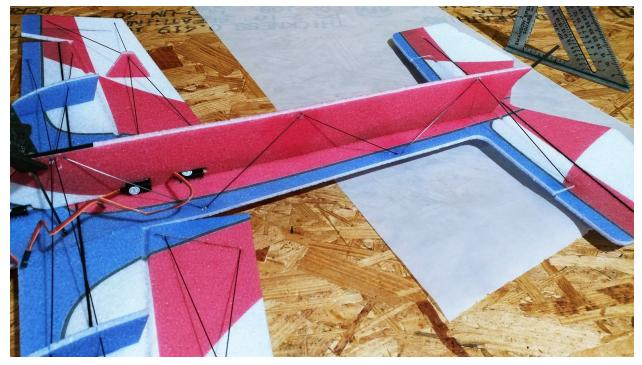
You can now brace along the underside of the fuselage. The 4 pieces that are the same length are 125mm. The long piece that extends from the fuselage to the horizontal stab is 155mm.
