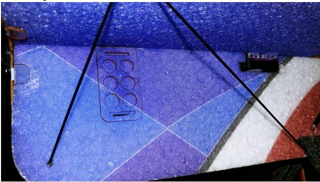
The plate shown above is used to assist with the mounting the electronic speed controller. The plate will be glued on the opposite side of the fuse of where the ESC will be mounted. You will find the mounting location at where the slots are cut in the fuselage. If needed, slightly enlarge the slots after the plate is glued. These slots will be guiding the velcro strap that is provided with the kit to mount the ESC.
