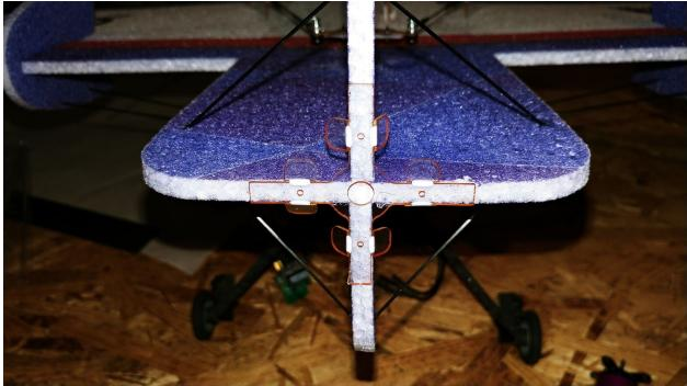
Locate the motor mount and make sure that all four ends of the mount line up to the indents made in the foam. Also when glueing on the mount as shown above, make sure is is pressed directly up against the foam and made flush. Next, bend the tabs over on each side 90 degrees and give them a hard press against the foam. You may wish to add glue to the tabs.
