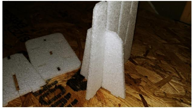
Provided in the kit is the EPP stand used to slide over the fuselage. Assembly is shown as above.
