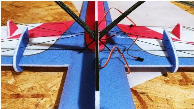
This 190mm flat carbon fiber piece will be used to strengthen the bottom of the fuselage from the front of the fuse through the landing gear location.
