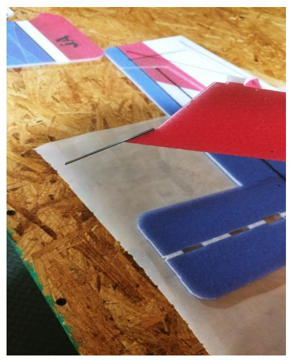
As shown in the photo above, a flat piece of carbon fiber will be used for the tailwheel purpose and allow the aircraft to rest and taxi on the ground without coming in contact with the foam. This will be glued to the bottom vertical piece of the fuselage. The length of this piece is 60mm.
