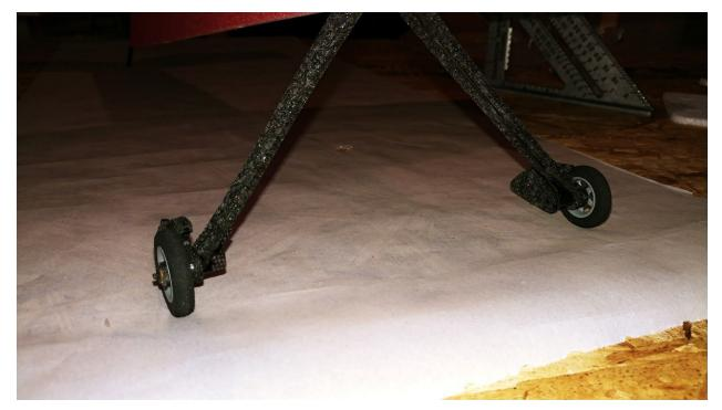
Now, you can apply the foam landing gear covers. Once you make sure that the carbon fiber rod of the landing gear is fully inserted into the slots, you can apply glue to the connection at the bottom of the cover as well as at the top where it joins the fuselage. Also, make sure to put glue along the landing gear to ensure the covers will stay flush.
