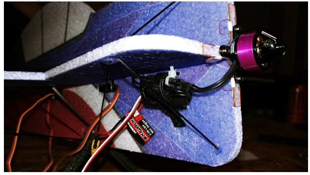
Shown above is the ESC side, the opposite side is where the plate was mounted. Notice the velcro strap coming through the fuselage and around the ESC. A small piece of velcro may be needed to mount the ESC directly on the foam as well for the best possible strength.
