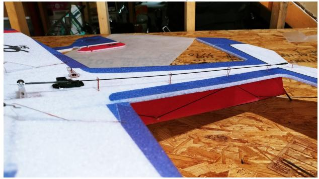
Once the servo is centered, and both sides of the linkage are glued and tightened with heat shrink, you can now glue in place the guides for the linkage. It is best to put a small bit of glue inside the cutout then place in the guide. Make sure that they are all standing straight up and flush with the fuselage. If the linkage is getting stuck in one of the holes, use sandpaper on the linkage to ever so slightly slim the carbon.
