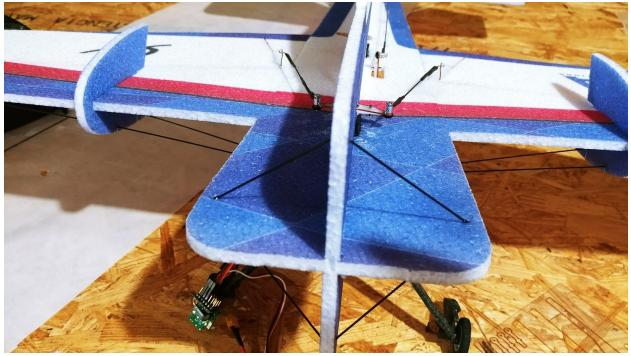
Once the top fuselage is fully glued in place, the bracing for the top can be started. Shown above are the two 80mm carbon rods used for forward bracing of the aircraft.
