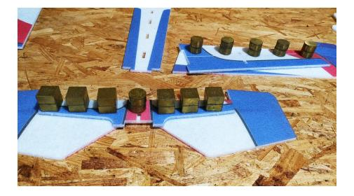
In order to get consistent full range of all control surfaces during flight and setup, we recommend that the first thing you do after unboxing is weighing down the control surfaces as shown above. Each surface will take about 60-120 minutes to complete, then you will notice that it will be easier to move the surface to full deflection.
