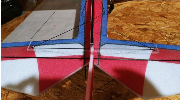
Now that the top part of the fuselage is glued in, you can finish the bracing for the bottom by including the 2 pieces that will connect the horizontal stab to the vertical stab aft of the tailpiece (behind the connection made when glueing the top of the fuse to the bottom). The 2 carbon rods are 160mm.
