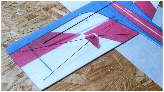
With the joiner in place, you can now begin the process of bracing the aileron. This will include four carbon fiber rods in the configuration shown above. The lengths for each are 190mm, 170mm, 140mm, and 155mm. The carbon rods will be pre-cut. You may also be able to spot the black dots where carbon can be referenced for placing. Be sure to provide a good connection for the carbon by poking through the foam.
