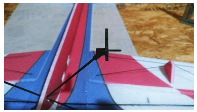
The wheel spat will be the first thing that is put on the axle. This will go all the way flush to the landing gear/axle joiner. Add a drop of glue to put this into place once it is positioned to your desire.
