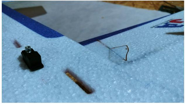
The control horns will be placed and glued into the slots of the appropriate control surfaces. Make sure when applying the control horns that they are flush and that the hole for the linkage is directly above the hinge line. It may be a good idea to scuff the sides of them with sandpaper. Shown above is one of the aileron control horns.
