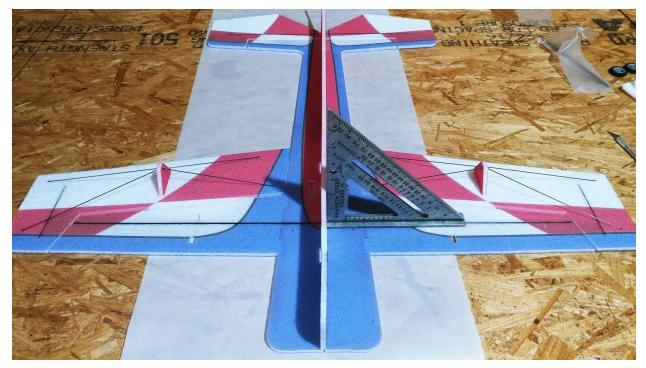
Making sure that everything is 90 degrees and flat, it is important to test fit the underneath side of the vertical fuselage. The fit should be fairly snug, so do not glue any spots until you know that each tab will be inserted fully along the fuse. Once this is complete, you can then apply glue along the edges. When placing back in, once again make sure that it is adjusted at 90 degrees to the rest of the airframe. There is no need to apply glue to the edges that will cover the servos.
