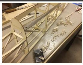
Glue the balsa nose blocks together and fill the voids in them with ballast weight.
