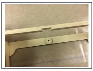
cut a notch in the ¼" stick to allow it to fit over the ring. Additional pieces of ¼" stick is added to the appropriate notches in the formers. Make certain that the angle of the formers is not changed as these pieces are added.
