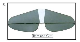
When cutting through the covering to remove it, cut with only enough pressure to only cut through the covering itself. Cutting into the balsa structure may weaken it. - Using a modeling knife, carefully remove the covering that overlaps the stabilizer mounting platform sides in the fuselage. Remove the covering from both the top and the bottom of the platform sides.
