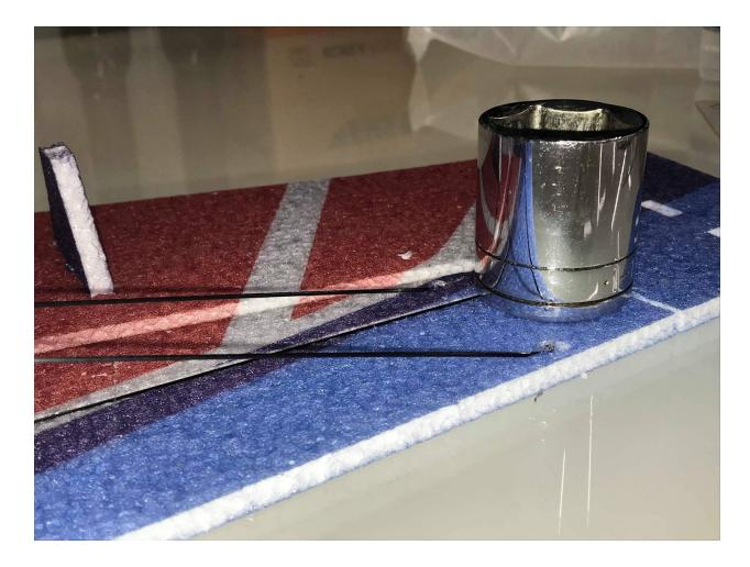
Just like the aileron bracing, it is very important to use weight towards the wing tip while the carbon wing bracing is setting to keep the leading edge of the wing as straight as possible.
