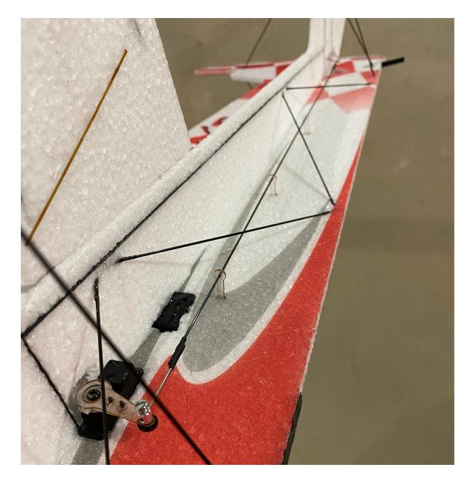
Above is the finished elevator linkage setup with the guides glued into the fuselage and the elevator centered and clamped into the mini EZ connector.
