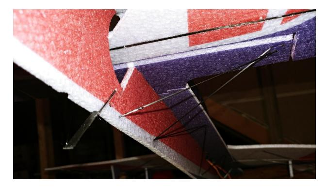
Now that the top of the fuselage is glued in, you can glue the other rear carbon fiber rods to help strengthen the tail as shown above. They will be mounted from the bottom of the horizontal tail to the rear of the bottom vertical fuselage. Make sure they are glued in a location that allows for full down elevator throw.
