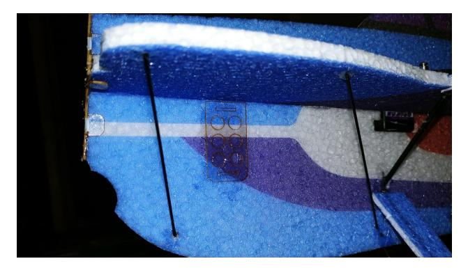
Notice above the plate glued onto the side of the fuselage. This can be used to mount the electronic speed controller on the other side of the fuselage. The two cutouts on the top and bottom of the plate is where the provided velcro strap will slide through.
