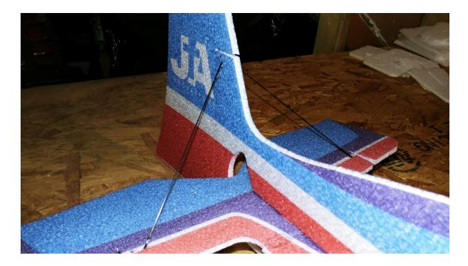
Shown above is the carbon rod that will go on each side of the fuselage. It will
