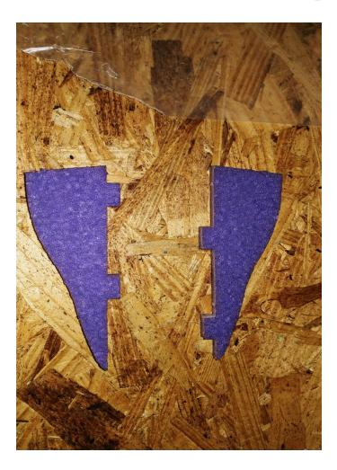
If desired, locate the side force generators that will be glued into the counterbalances of the ailerons. \*Some airframes may require the SFGs to be glued into different locations along the wing.\*
