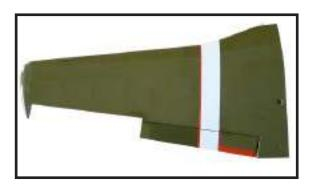
Note: Work the flap up and down several times to "work in" the hinges and check for proper movement.
