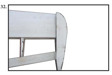
Locate and assemble W12 (wing tip) by epoxy glue as photo shown (photo 30).
