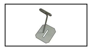
2) Remove each hinge from the wing panel and flap and place a T-pin in the center of each hinge. Slide each hinge into the wing panel until the T-pin is snug against the wing panel. This will help ensure an equal amount of hinge is on either side of the hinge line when the flap is mounted to the wing.
