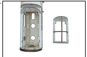
Attach the plastic pushrod tube to the pushrod hole at each former fuselage as photo shown (photo 59).
