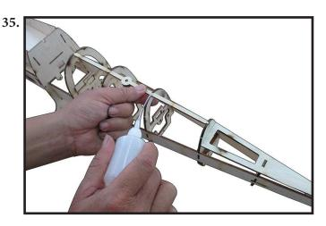
Locate and assemble F19 to fuselage by CA glue as photo shown (photo 36).
