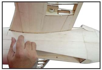
Use the paper blade cut down and use sanding tool to make flat and seamless from the fuselage to the bottom of wing (Photo 6).
