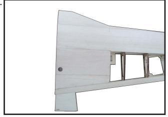
Reinforced W37 to sheeting at the wheel area as photo shown (photo 25,26,27). Then, step by step cover sheet one after another in order W31-W33-W35-W38 for top of wing.
