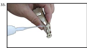
Locate and assemble F22 to fuselage by CA glue as photo shown (photo 34).
