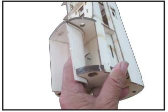
Locate and apply the sheet SH6 to fuselage (left side and right side) by CA glue as photo shown (photo 75).
