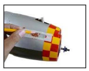
4) Slide the muffler screws through the engine. Place the mufflr extension and gaskets included with the engine on the screws. Be careful when mounting the cowl so the screws and extension remain in position until the mufflr can be attached.
