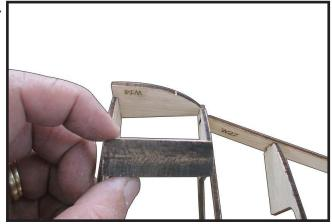
Locate and assemble lock wing tube (W18) as shown photo (Photo 12).
