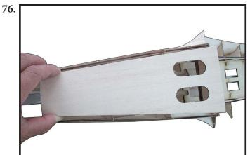
Locate and apply double 8mm balsa F8A to fuselage (left side and right side) by CA glue as photo shown (photo 77).
