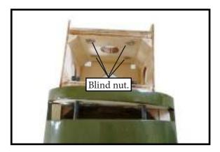
5) Attach the motor to the front of the electric motor box using four 4mm blind nut, four M3x15mm hex head bolts to secure the motor. Please see picture shown.
