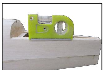
Assemble the triangle balsa block and cut down the excess part to rounded shape like T1 at intersect place. Then, sanding around it until it look like seamless with the end of fuselage (Photo 2,3,4,5).
