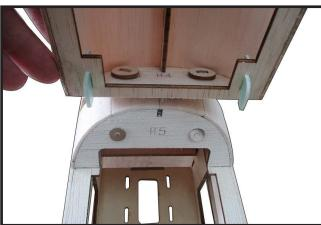
Setup the hatch and the fuselage so that the top of hatch seamless the top of fuselage by sanding tool (photo 86).
