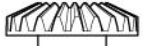
MC13 ×4 51008 ベベルギヤ (大) Large bevel gear Kegelrad groß Grand pignon conique
