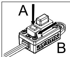
1. Connect a battery. Press and hold the set button and turn on ESC. The RED LED will flash.
