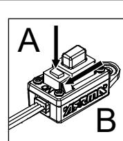
4. Switch off ESC to complete setup
