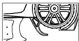
1. Throttle trigger in neutral position - press set button (1 Green flash)
