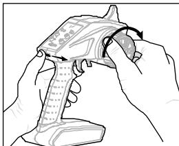
Turn the steering wheel to Full Right. Power the transmitter on while holding the steering wheel to the Right.
