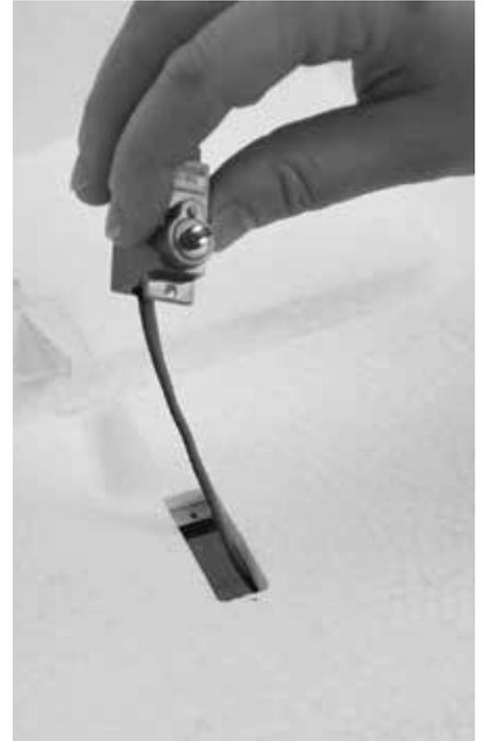
**TIP:** Plug a spare servo extension into the servo lead before removing to make it easier to install the lead of the servo when replaced.
