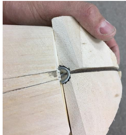
Next glue in nose formers and blocks. Not to allow a cavity for nose release wire loop. Then sand nose blocks to shape using the guide formers as reference.
