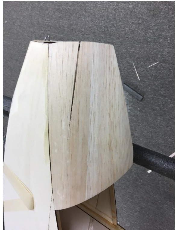
Next glue in nose formers and blocks. Not to allow a cavity for nose release wire loop. Then sand nose blocks to shape using the guide formers as reference.
