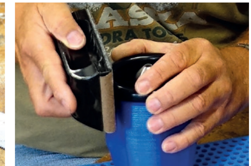
69. Abflachung parallel zur Impeller-Gondel schleifen. / Flatten parallel to the impeller gondola grind.
