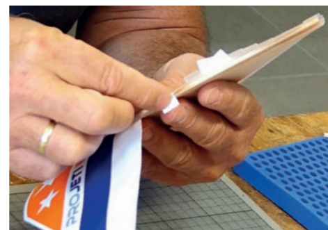
105. Überlappungen von hinten beginnend in Flugrichtung aufkleben (Keine Stöße in Flugrichtung). / Place the overlaps from the back in the direction of the flight (no impacts in the direction of flight).
