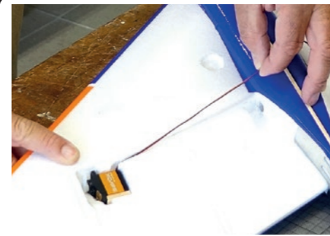
37. Servokabel in Kabelkanal einlegen. / Insert the servo cable into the cable channel.
