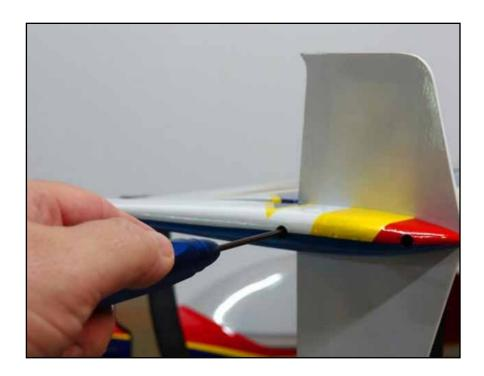
TEMPORARY NOTE: The first few shipments of 69" Raven v2 have a mislocated hole in the clear plastic wingtip, this will be corrected on later shipments, you may need to drill the rear hole as shown to correct.
