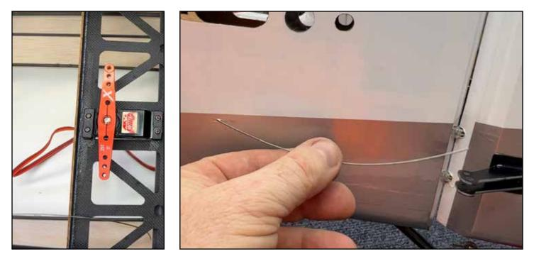
To terminate the cables at each end, you will use a ball link, a brass threaded end, and the small metal crimp tube. Thread the ball link onto the brass threaded end, and attach to the servo arm and control horn with screws, washers, locking nuts and cone spacers as applicable.
