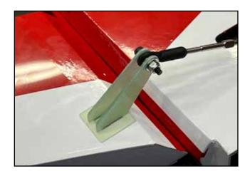
Apply good quality 15 or 30 minute epoxy into the slots and to the scuffed area of the horn. Press the horn firmly into the slot and make sure it seats all the way. Clean up any excess epoxy with a rag and denatured alcohol.
