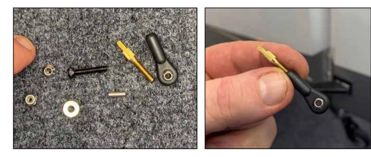
To attach the cables, lace them through the crimp tube and brass end in the pattern shown. Pull the cable snug (not banjo-string tight) and crimp the tube with pliers to lock the cable in place, and drip one small drop of thin CA into the crimp tube.
