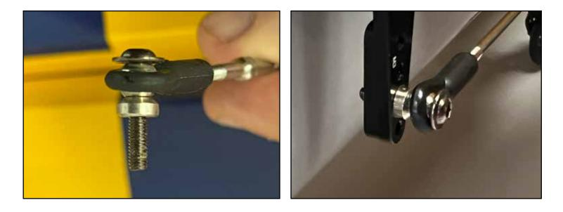
Mount the aileron servos as shown, using a servo wire extension as needed. Look closely at the linkage, this is how the linkage should appear with the servo centered and the pushrod set to the correct length.
