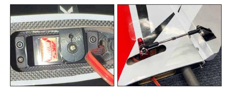
On many linkages, a cone-shaped spacer is included if needed. This spacer goes between the ball link and the servo arm to prevent any interference between the ball link and arm. The pushrod has one left-hand and one right-hand threaded end. This allows you to spin the pushrod to change its assembled length after installation.
