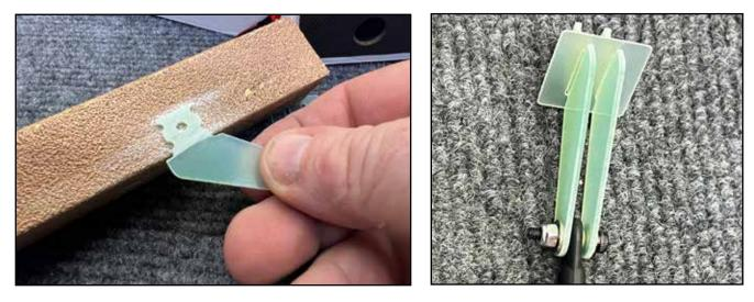
Locate the slots in the control surface, remove covering as shown with a hobby knife. Test fit the horn into the surface, make sure it seats fully. If necessary, remove any sawdust or debris from the slot.
