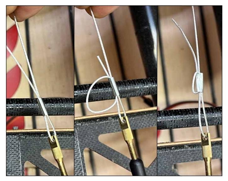
After installation, you can tighten or loosen the cables as needed for maintenance by rotating the brass threaded ends to screw them into or out of the ball joints.
