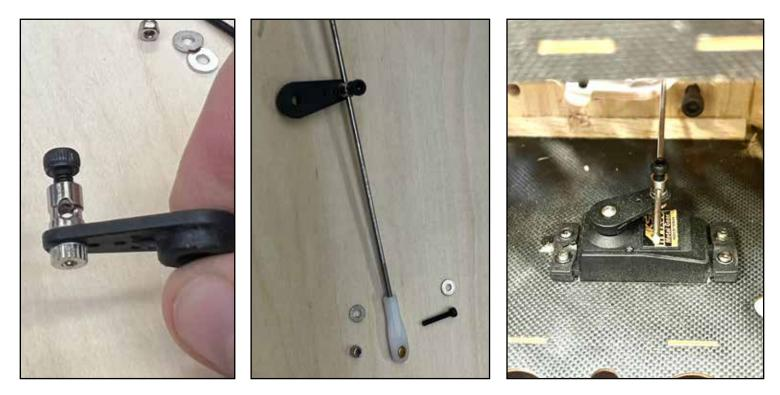
If your engine and its carburetor and throttle arm allows it, it is an upgrade to use a 1" metal servo arm on the throttle servo, and to use a throttle pushrod with ball links at each end. Pictured is a typical twin-cylinder throttle installation, with the throttle servo on the outisde/bottom of the motor box.
