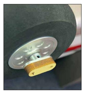
Install the wheel pant over the wheel and axle, tighten to the landing gear with one or two screws as designed, using blue loctite. The wheel pant support should sit against the pant as shown. Flex the pant away from the retainer and apply some epoxy glue between the rainter and pant.
