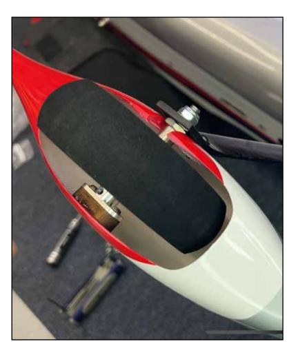
The 85" Yak uses a half-pant on its wheel. To install these, drill holes as appropriate for the wheel axles, and sandwich the halfpant between the axle and landing gear as shown. Lock the half-pant in place with included wood screws as shown. Finish with a wheel collar to retain the wheel, use blue loctite on the set screw.
