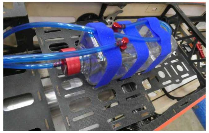
Locate your fuel dot in the fuselage side as shown. Mount your ignition to the motor box as shown, and arrange power for your ignition. We prefer an IBEC, such as the Tech-Aero IBEC unit.
