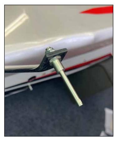
Most Extreme Flight aircract use full-coverage wheel pants (The 85" Yak is one exception) and so they have a wheel pant support integrated into the outer wheel retainer. Assemble the retainer from the wood piece and aluminum piece with screws as shown. Place the wheel on the axle and retain with this assembly. Use blue Loctite on the set screw.
