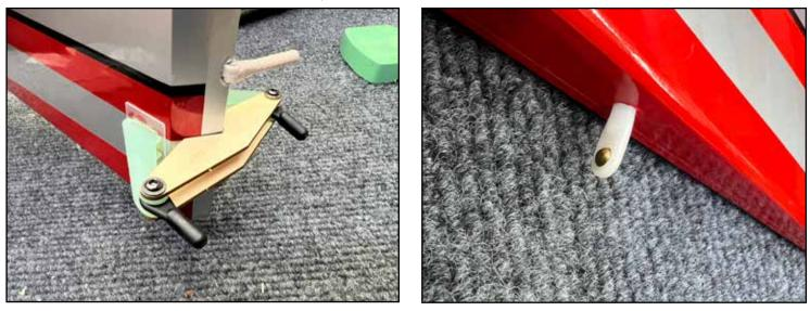
Apply a bit of petroleum jelly (vaseline) to the center of the rudder hinge points to protect the hinge mechanism from glue, and glue the hinges into the fuselage using 15 or 30 minute epoxty. Clean up any excess epoxy with denaturted alcohol. Use masking tape to hold the rudder perfectly in position while the glue cures.
