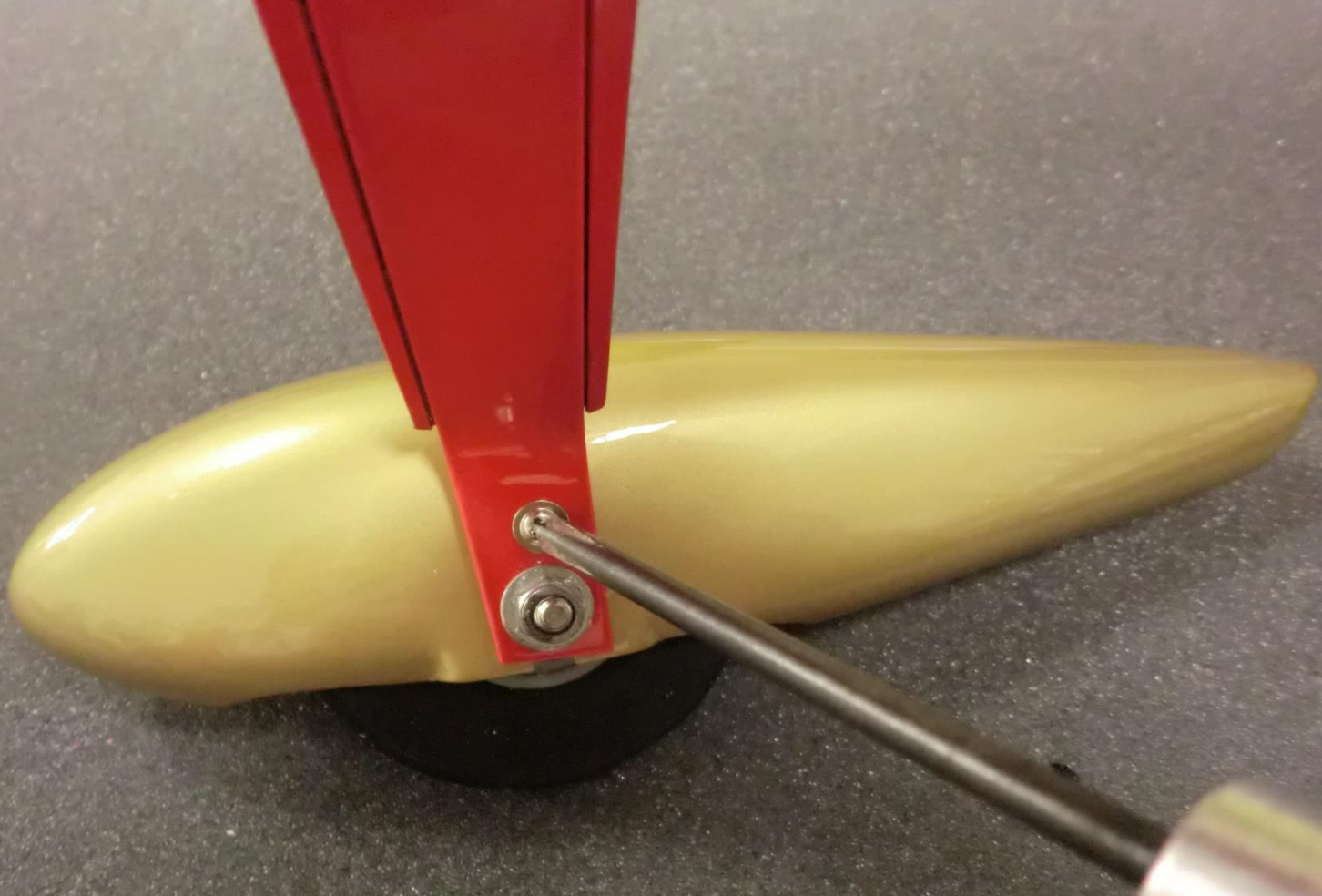
Landing Gear installation
