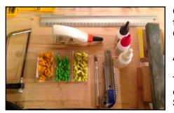
Craft Knife or Scalpel, 120 + 240 grit sand paper (supplied in the kit), fine saw, Modelling pins, Clothes-pegs and clamps.
