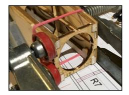
Glue the two Balsa rings R1C-28 and R1D-28 together.
