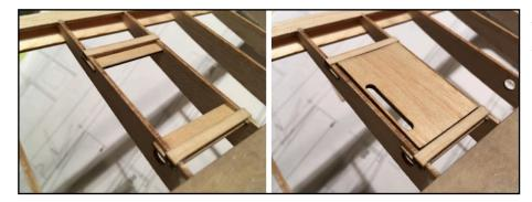
At the bottom, the holding screw reinforcement bars for the servo box hatch cover are now inserted into the slots pre-cut in ribs 9 and 10. Using the hatch cover as a template, make a frame from scrap 2mm Balsa for the hatch as shown for attaching the covering film to.
