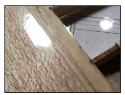
After that, the flap is swung back into the neutral position. Revealing a fine gap where the film is just visible.
