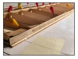
The trailing edge is completed by the **Poplar ply** strip **EL-2.1**. This is glued to the lower sheeting, the ribs and the top sheeting (oben) as shown in the picture.
