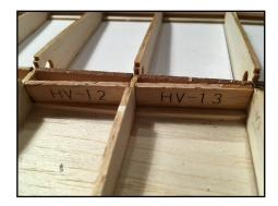
The reinforcement gussets **3-4** and **16-19** are glued to the false leading edge. **3-4** fits halfway through rib **3**!
