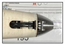
Using some scrap **0.4mm Ply**, you can make an air scoop to go over the motor cable slot. Alternatively you can make a flush cover if you prefer.
