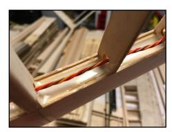
Once you have achieved a good fit between the inner panel joiner **HVB** and the middle panel web **HV-2** and a clean transition between the two panels, glue, pin, and clamp the two end ribs **17** and **18** together with Epoxy and fill the gap between the upper and lower spar caps between ribs **18**, **19** and **20** with Epoxy as shown in the picture.
