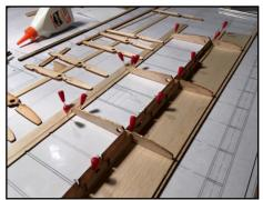
The wing joiner strip **HVB**, is integrated with the inner panel before fitting rib **16** and **17**. The remaining ribs are then added. The easiest way is to slot all the ribs in position and then glue them in place. The root block (ribs **2** and **3**) and end
