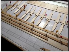
Release ribs **2-17** from their carrier sheets and using them as templates to ensure it is positioned
