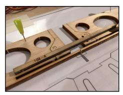
Round off the leading edge of the horizontal stabiliser. Carry out the same procedure with the fin and rudder with the bevel on the rudder on the control horn (right) hand side!
