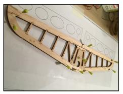
Laminate the elevator connecting strip from parts **2 x HR-4** with glue and then glue it into the slot in the elevator. Sand a 30° bevel on the bottom leading edge of the elevator and a taper on the trailing edge as shown on the plan.
