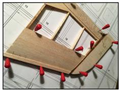
When everything has cured, cut any excess capping strip or sheeting flush with ribs **34** and **37** before gluing the end rib **38** in position.
