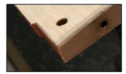
Sand an oblique angle to the trailing edge (see picture) where it sits on the wing mounting plate **R6-1**, so that the wing panel slots easily in place on the fuselage. See the plan for detail.
