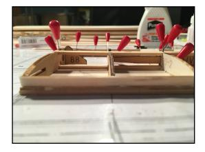
Note: Take care when positioning web HV-2 on the spar cap, because the spar joiner HVB protrudes two rib fields into the middle panel – up to rib 20!
