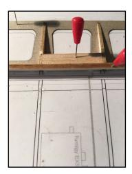
The **3mm Balsa** leading edge (**QR-1**) is then pinned on the ribs and bottom sheeting before being glued in place.
