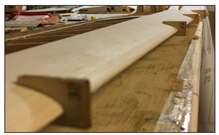
As previously mentioned, the wing panels are glued together from the outside to the inside. I.e. Wingtip onto Middle panel using PVA or Epoxy. Then middle panel onto the inner panel using 30 minute Epoxy.
