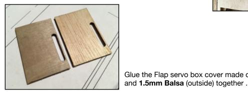
Glue the Flap servo box cover made of **0.4mm Ply** (inside)
