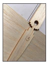
Remove the **1.5mm Balsa** wing underside panels from the carrier sheets and pin them on the plan and glue them together.
