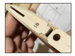
Next comes the **2x3mm Pine** trailing edge reinforcement spar, which is inserted into the recesses at the back of the ribs and glued.
