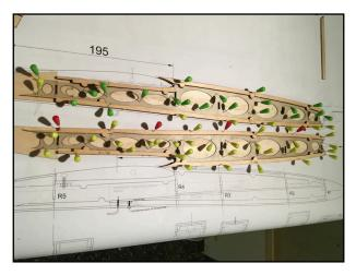
Pin the fuselage side walls together over the plan and glue with CA or PVA.
