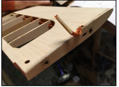
The 1.5mm Ply end Rib 1 is glued in place only after the servo cables have been pulled through. Servo cables of the required length are included in the kit.
