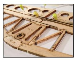
Note: Don't forget to remove the covering film from the gluing area before gluing the fin in place!
