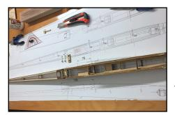
Now put the second fuselage side wall on the formers and make sure they are all fully located in their slots. Clamp them together but. **Don't glue anything together yet!!**
