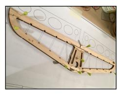
Assemble the horizontal stabiliser from parts **HL1** - **HL9** and the elevator halves from parts **HR1** -**HR 3** and pin them to the plan, and glue together with Medium CA or PVA.
