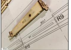
Glue the doubler **R11** to the Stabiliser mounting plate **R11.1** and glue the **M3** plastic nut into the prepared opening.
