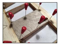
Likewise, the **0.4mm Ply** covering of the flap servo box is now also glued in place.
