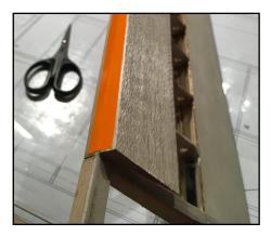
In this case, using a credit card, or similar (I use a metal rule) as a spacer, the flap is laid upside down on the underside of the wing flush with trailing edge.
