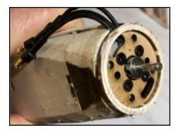
Glue the Balsa ring onto the motor plate.
