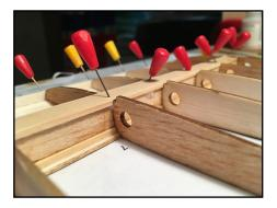
Glue the **3mm Carbon incidence pin** into the wing root as shown on the plan.
