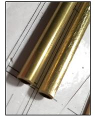
Roughen up the Brass wing-joiner tubes and slide them into the precut holes in the ribs. Tack them in place with medium CA before filling the void around the tubes and between the front and rear spar webs with Epoxy Resin as shown.
