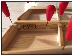
Pin and glue the **4x20mm Balsa** trailing edge in position against the back of the ribs.
