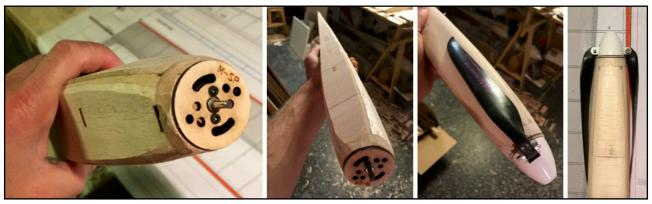
After the glue has set hard, the fuselage is ready for finishing and can be sanded to shape. Depending on the desired appearance and desired look, the edges can be rounded, as shown in the sectional drawings.
