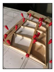
Glue ribs **34** to **37** in position over the lower spar cap and bottom sheet. The dihedral angle of rib **34** is set by the spar web **HV-3**, in the first rib bay.
