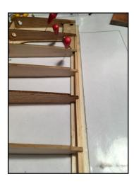
The **2x3mm Pine** reinforcing strip is threaded into the slot in the back of the ribs **4-17** and glued in place.
