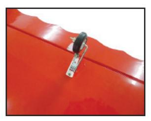
3) Hold the rudder in place and mark it where the music wire will enter. When you are happy with the fit, fill the hole with epoxy and use CA to glue in the rudder hinges.
